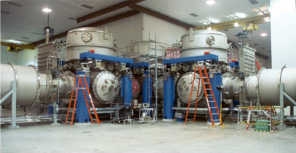
Figure 3-3: Photo of the L1 vacuum system vertex in the LIGO Livingston Observatory corner station (Courtesy LIGO Laboratory).
