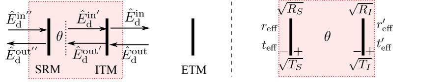
**Figure 2.14** – Mapping from a three-mirror cavity to a two-mirror cavity by defining the effective transmissivities ( $t_{\text{eff}}, t'_{\text{eff}}$ ) and reflectivities ( $r_{\text{eff}}, r'_{\text{eff}}$ ) of the signal-recycling cavity.
