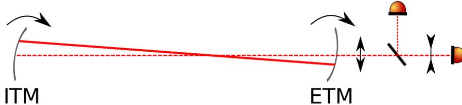
Figure 2.6: Sensing of Fabry-Perot cavity axis motion using two QPDs in transmission.
