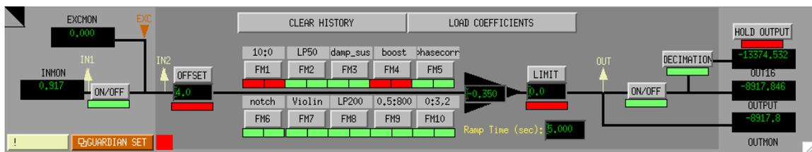
Figure B.2: DARM filter bank. Algorithm downloads input signal and computes output using two types of variables to estimate quantization noise of digital filters that are engaged.
