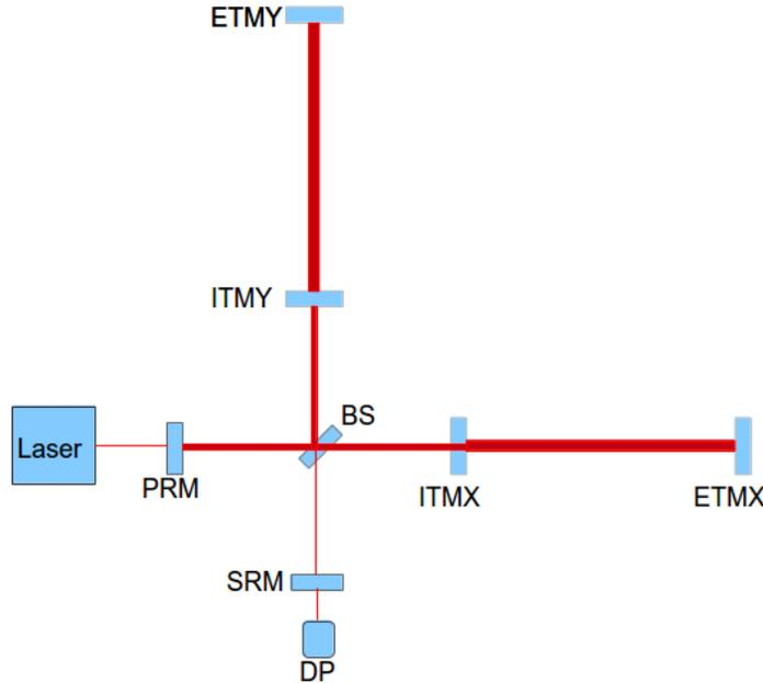
Figure 1: Schematic of interferometric detectors, like LIGO.
