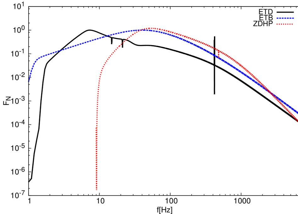
Figure 26: The panel shows the expected sensitivity for two configurations of the Einstein Telescope (ET), namely, ETD (black), ETB (blue) and LIGO’s Zero Detuned High Power (ZDHP) configuration (red). The vertical axis measures  $F_{\text{normalized}} = (f/f_{\text{max}})^{-7/6} \sqrt{S_n(f_{\text{max}})/S_n(f)}$ , where  $f_{\text{max}}$  is the maximum of the corresponding power spectral density,  $S_n(f)$ .
