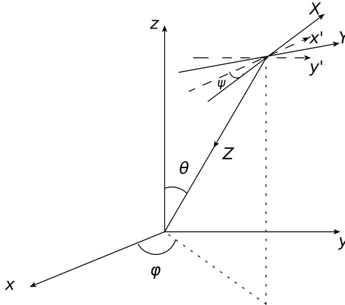
Figure 2: The angles  $\{\theta, \phi\}$  show the relative orientation of the radiation  $(X, Y, Z)$  and the detector  $(x, y, z)$  frames.  $x'$  and  $y'$  axes are parallel to the  $x$  and  $y$  axes, respectively.  $\psi$  is the angle by which the radiation frame is rotated, around the line of sight.
