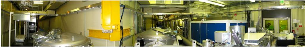
Figure 4.2: Panorama picture of the 40-meter prototype facility. The picture was taken from the corner of the Michelson interferometer. It shows the  $x$ -arm vacuum tube on the left,  $y$ -arm vacuum tube in the middle, and the main laser booth (the one with blue doors) on the right of the picture.
