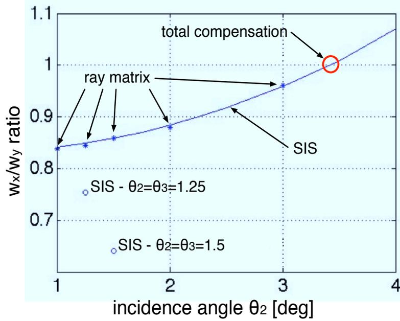
Figure 6.21: Simulation of astigmatism of radio-frequency sidebands in the *vertical* layout: the plot shows the ratio  $w_x/w_y$  versus  $\theta_2$ , computed for  $\theta_3 = 1$  deg with the ray-matrix code (stars) and SIS (blue curve), and for  $\theta_3 = 1.25$  deg and  $\theta_3 = 1.5$  deg with SIS (empty circles), from [107].
