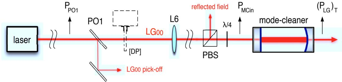
Figure 8.41: Measurement of the  $LG_0^0$  beam through the experimental setup. The usual position of the diffractive plate (DP), removed from the setup for the measurement of the transmission, is shown with a dashed line.
