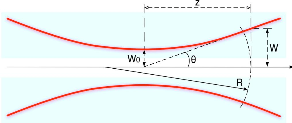
Figure 5.1: Parameters of a Gaussian beam.
