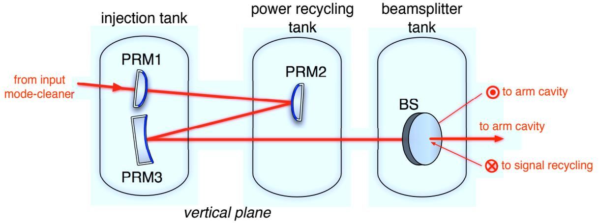
Figure 6.19: Layout of *vertical* non-degenerate recycling cavities.
