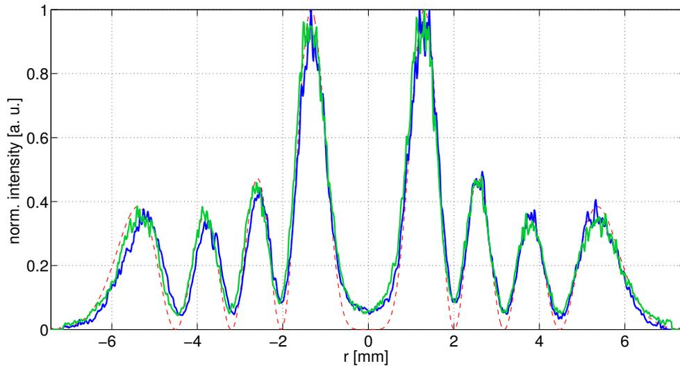
Figure 8.39: Profile comparison: the horizontal (blue solid curve) and the vertical (green solid curve) measured cross sections of the transmitted  $LG_3^3$  mode are shown, together with the cross section of the simulated theoretical  $LG_3^3$  mode (red dashed line). The theoretical mode is not a fit, but it is obtained by propagating the  $LG_3^3$  eigenmode of the mode-cleaner in space.
