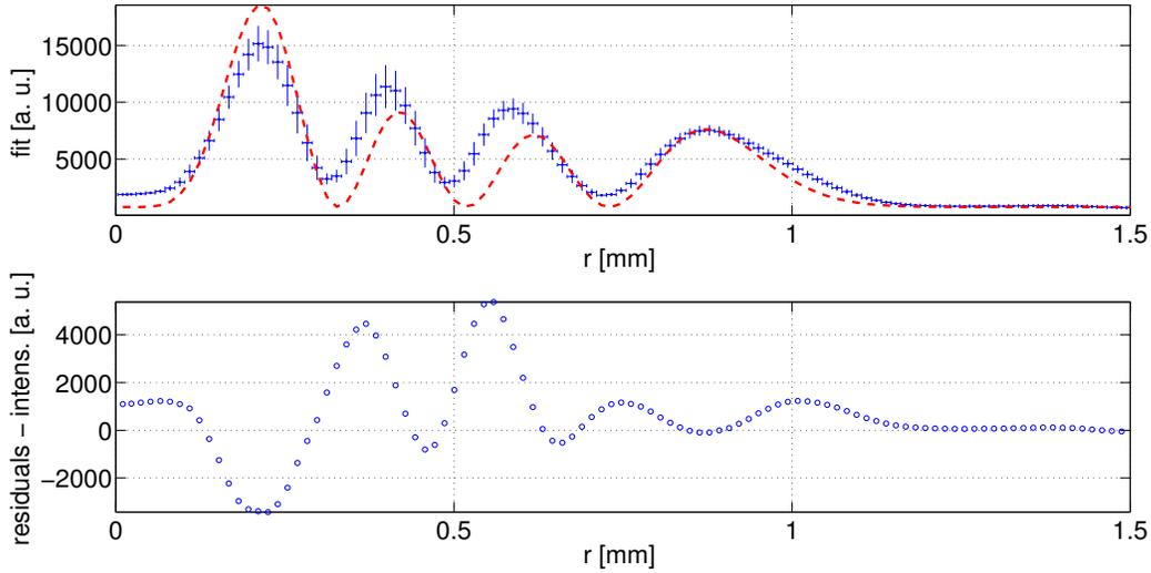
Figure 8.29: Least square fit of the pseudo-LG<sub>3</sub><sup>3</sup> mode profile. Top panel: measured (blue dots with errors) and fitted (red dashed curve) profiles in the  $r > 0$  plane. Bottom panel: fit residuals, defined as the difference between the data and the model.
