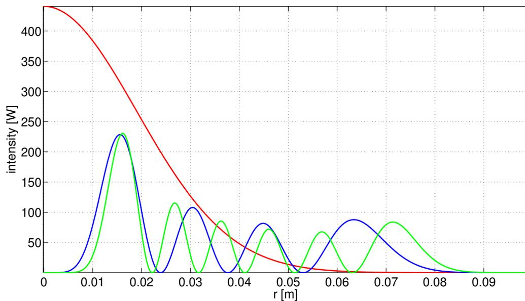
Figure 7.2: Intensity profiles of  $LG_0^0$  (red curve),  $LG_3^3$  (blue curve) and  $LG_5^5$  (green curve) modes versus the radial coordinate  $r$ , for a beam power  $P = 1$  W and for 1 ppm clipping loss on a mirror with 10-cm radius.
