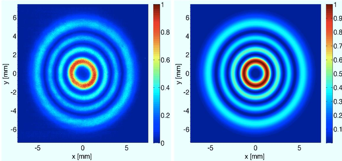
Figure 8.38: Comparison between normalized intensity distributions in far field: measured LG<sub>3</sub><sup>3</sup> mode (left) and simulated theoretical LG<sub>3</sub><sup>3</sup> mode (right).
