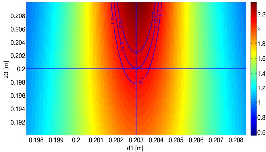
Figure 8.21: Tolerances of the telescope lengths:  $d_1$  [m] and  $z_3$  [m] are shown on the  $x$  and the  $y$  axis, respectively, and the vertical/horizontal lines represent the baseline values. The color scale indicates the size of  $(w_0)_{L3}$  [mm], the contours show the region for a change of the waist size of  $\pm 0.05$  mm.
