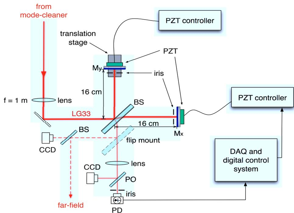
Figure 8.42: Layout of the Michelson interferometer illuminated with  $LG_3^3$  beams.
