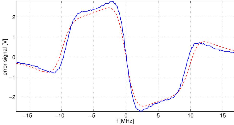
Figure 8.35: Pound-Drever-Hall signal of the pseudo-LG<sub>3</sub><sup>3</sup> mode: measured (blue solid curve) and expected (red dashed curve) signals.
