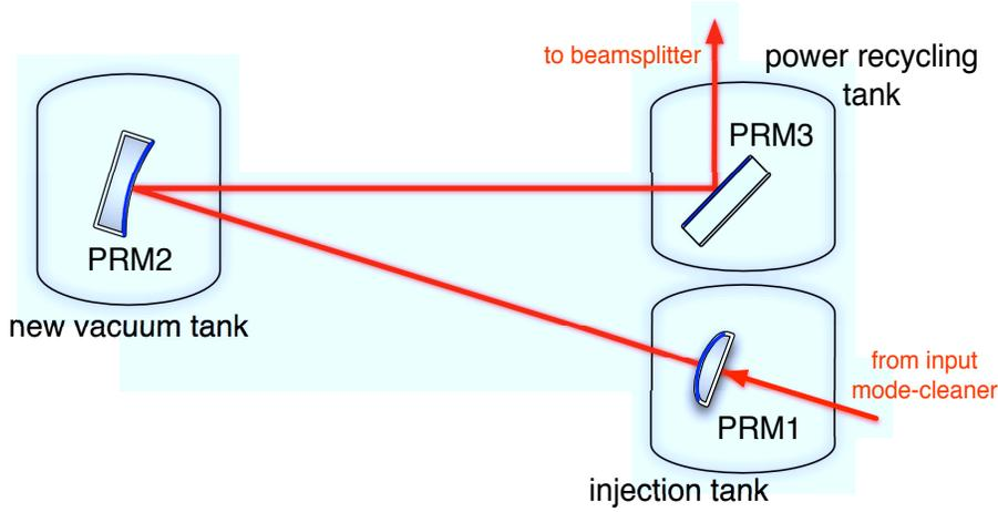
Figure 6.15: Layout of *long* non-degenerate recycling cavities.
