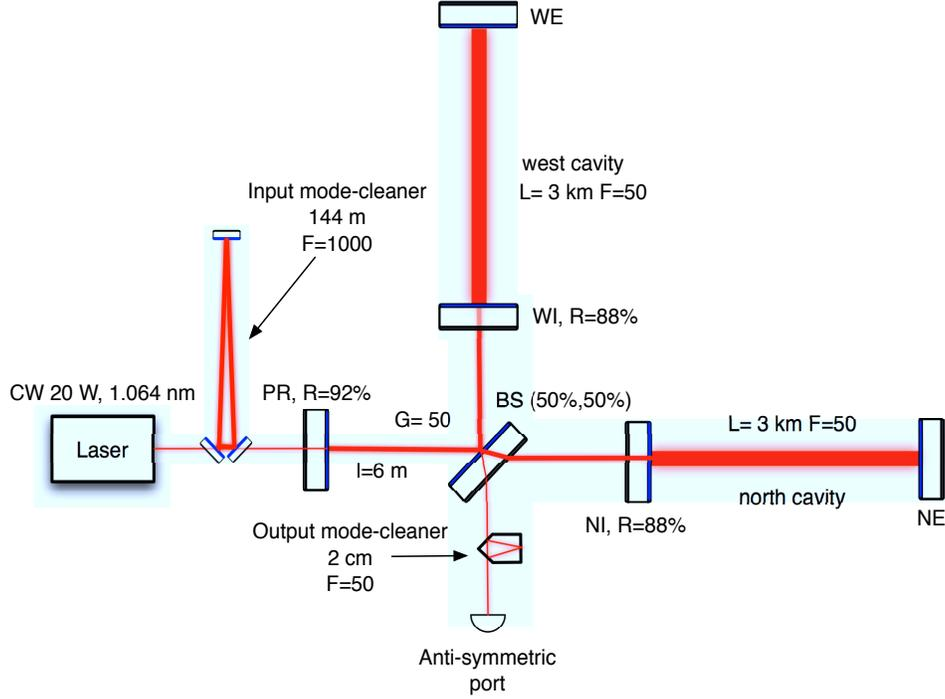
Figure 3.4: Optical layout of the Virgo interferometer.
