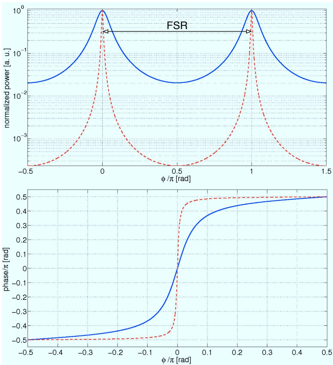
Figure 2.8: Normalized transmitted power (top) and phase of the transmitted field (bottom) of a Fabry-Perot cavity with  $L = 1$  km, no loss,  $r_1 = r_2$ , for  $\mathcal{F} = 10$  (blue solid curve) and  $\mathcal{F} = 100$  (red dashed curve).
