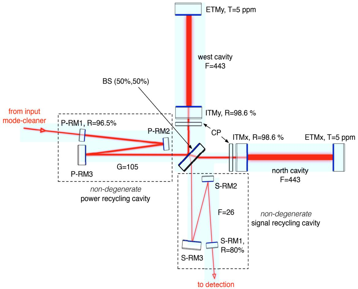
Figure 4.1: Optical layout of the Advanced Virgo interferometer.
