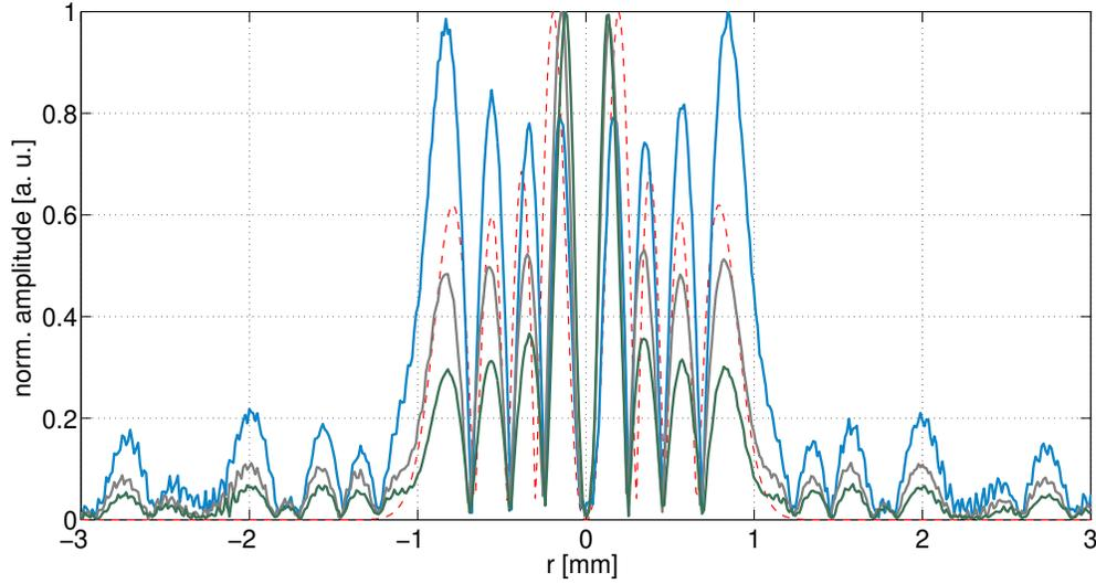
Figure 8.9: Normalized amplitude profile of the simulated pseudo- $\text{LG}_3^3$  mode, as a function of the Gaussian input beam waist:  $w_0 = 1.65$  mm (light blue curve),  $w_0 = 2.15$  mm (reference value, grey curve),  $w_0 = 2.65$  mm (dark green curve). The profile of the theoretical  $\text{LG}_3^3$  mode is also shown for comparison (dashed red curve).
