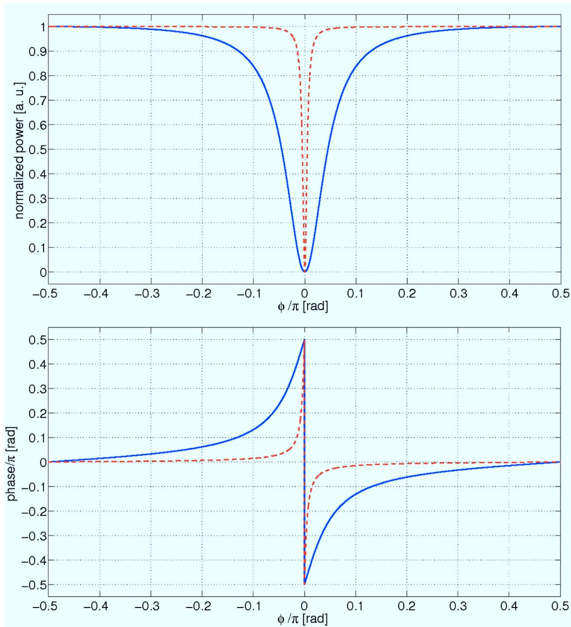
Figure 2.10: Normalized reflected power (top) and phase of the reflected field (bottom) of a Fabry-Perot cavity with  $L = 1$  km, no loss,  $r_1 = r_2$ , for  $\mathcal{F} = 10$  (blue solid curve) and  $\mathcal{F} = 100$  (red dashed curve).
