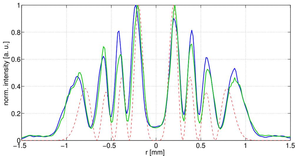
Figure 8.28: Profile comparison: the horizontal (blue solid curve) and the vertical (green solid curve) measured cross sections of the pseudo- $LG_3^3$  mode are shown, together with the cross section of the theoretical  $LG_3^3$  mode for  $w_0 = 288 \mu\text{m}$  (red dashed curve).
