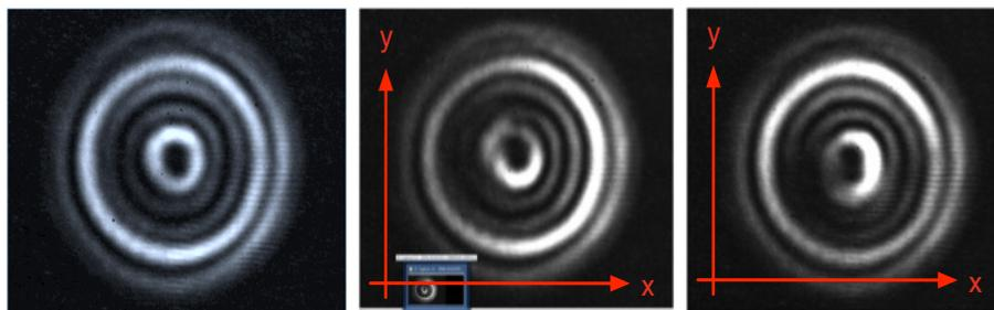
Figure 8.31: Field reflected by the mode-cleaner at the resonance of the  $\text{LG}_3^3$  cavity eigenmode: aligned field (left),  $x$  misalignment (center),  $y$  misalignment (right). The reference frame on the transverse plane is shown by the red axes.
