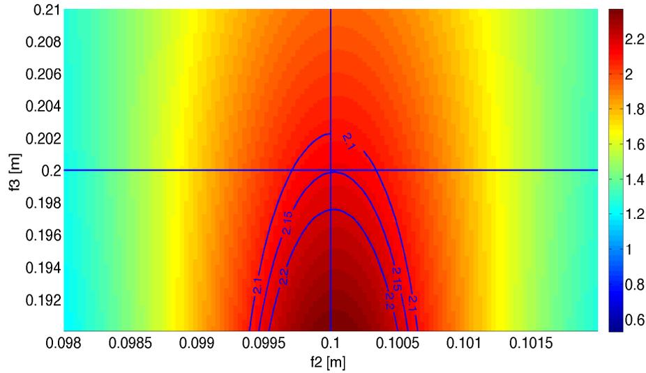
Figure 8.20: Tolerances of the telescope focal lengths:  $f_2$  [m] and  $f_3$  [m] are shown on the  $x$  and the  $y$  axis, respectively, and the vertical/horizontal lines represent the baseline values. The color scale indicates the size of  $(w_0)_{L3}$  [mm], the contours show the region for a change of the waist size of  $\pm 0.05$  mm.
