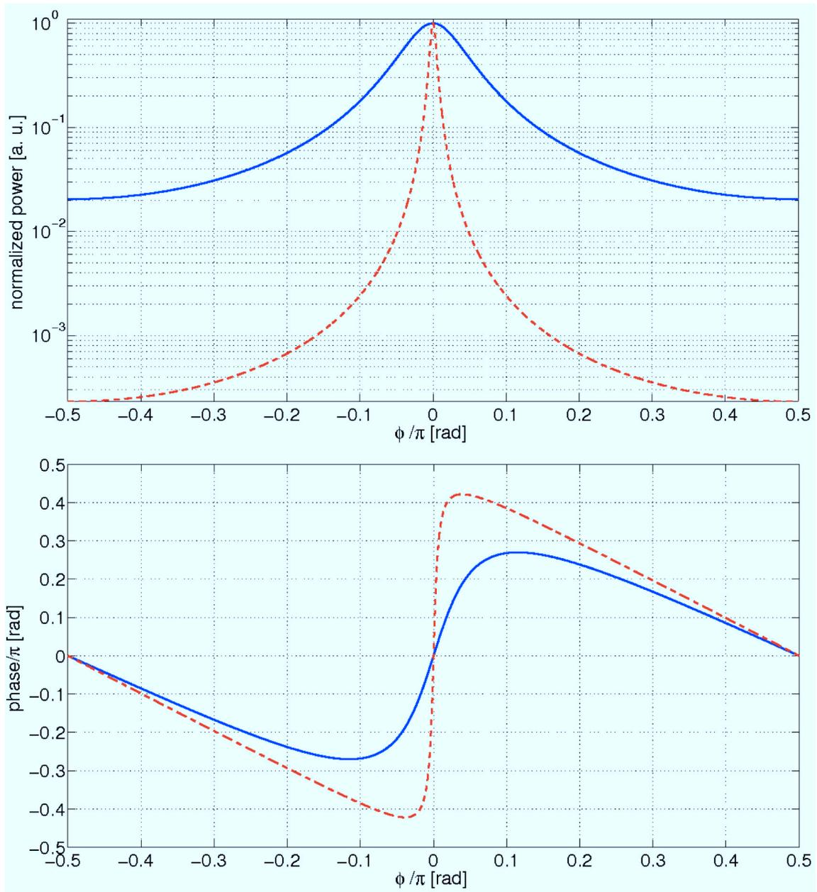
Figure 2.9: Normalized resonant power (top) and phase of the resonant field (bottom) of a Fabry-Perot cavity with  $L = 1$  km, no loss,  $r_1 = r_2$ , for  $\mathcal{F} = 10$  (blue solid curve) and  $\mathcal{F} = 100$  (red dashed curve).
