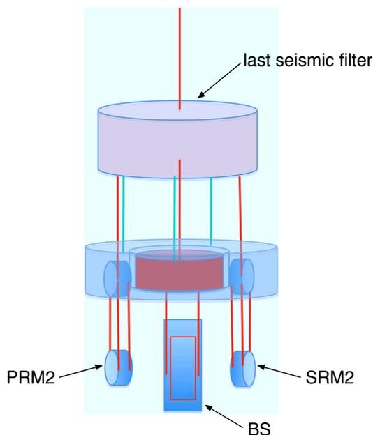
Figure 6.8: Scheme of the beamsplitter multi-payload, from [106].
