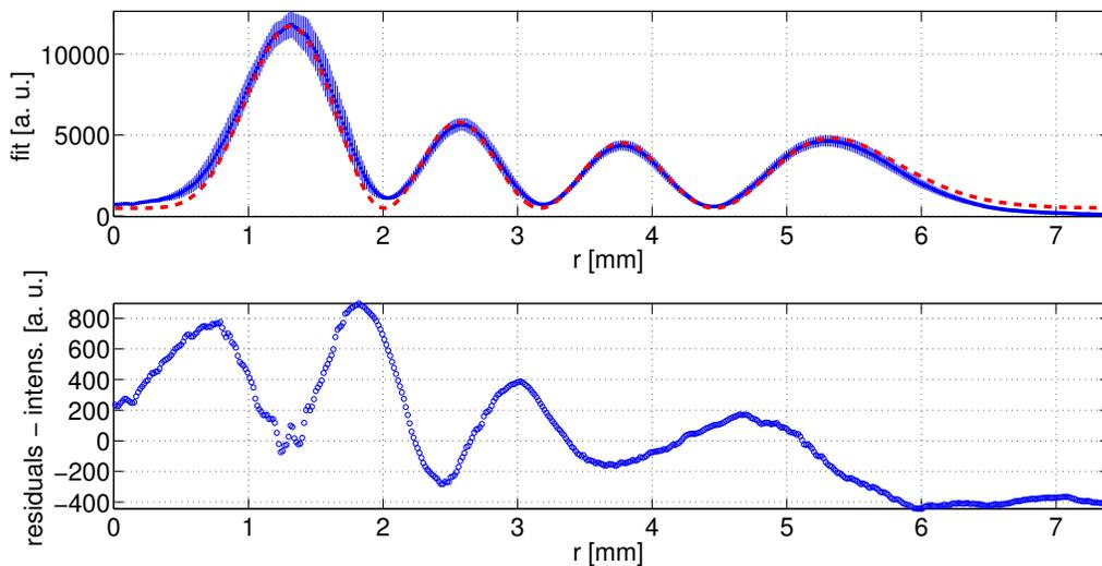
Figure 8.40: Least square fit of the profile of the transmitted  $LG_3^3$  mode. Top panel: measured (blue dots with errors) and fitted (red dashed curve) profiles in the  $r > 0$  plane. Bottom panel: fit residuals, defined as the difference between the data and the model.
