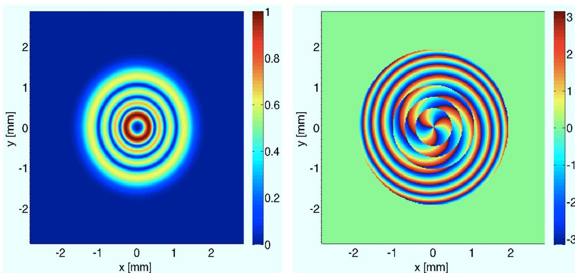
Figure 8.13: Theoretical LG<sub>3</sub><sup>3</sup> eigenmode transmitted through the mode-cleaner, for  $\mathcal{F} = 100$ : normalized amplitude [a.u.] (left) and phase [rad] (right).
