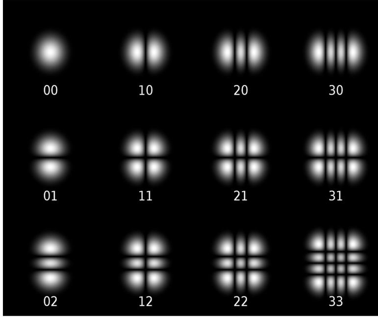
Figure 5.3: Transverse intensity patterns of  $\text{HG}_{mn}$  modes, from [97].
