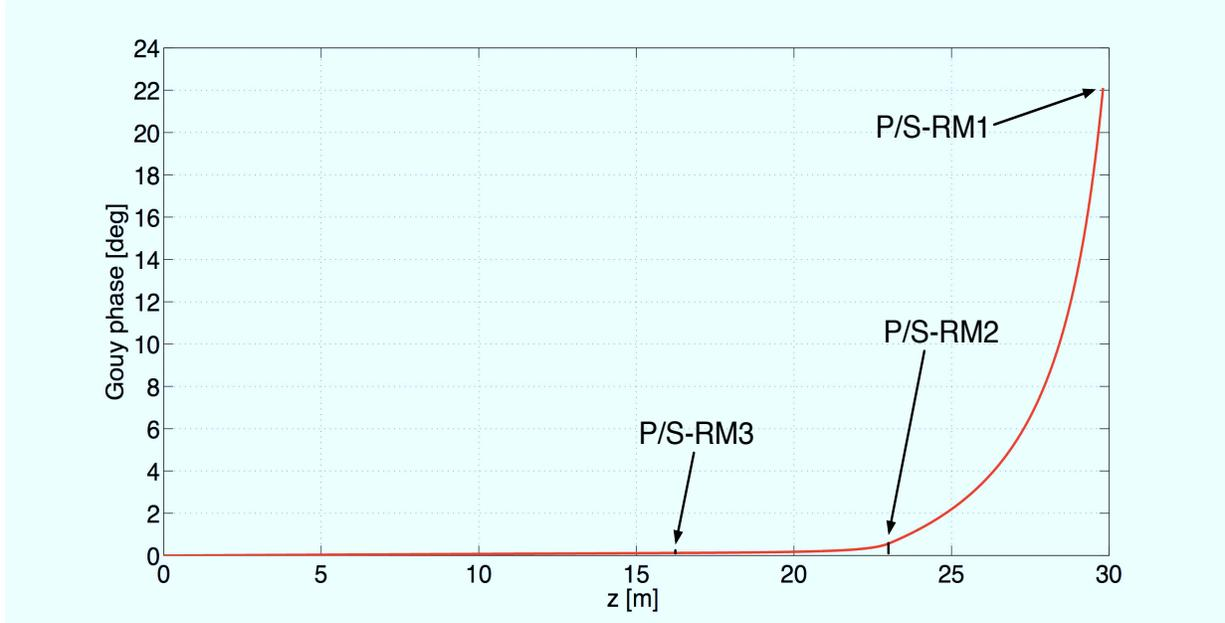
Figure 5.10: Evolution of the Gouy phase inside the non-degenerate layout.
