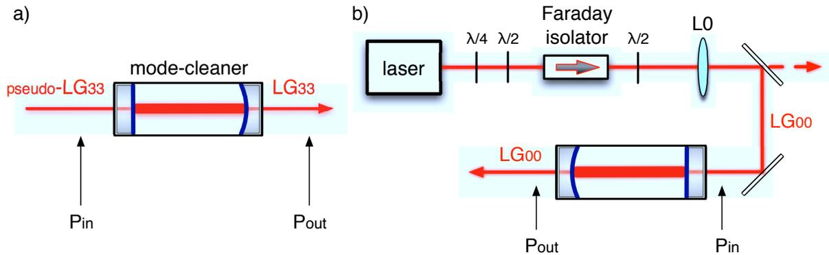
Figure 8.37: Setup for the measurement of the  $LG_3^3$  mode power transmitted by mode-cleaner cavity: a) transmission of the  $LG_3^3$  mode, b) characterization of the cavity throughput with the  $LG_0^0$  Gaussian beam.
