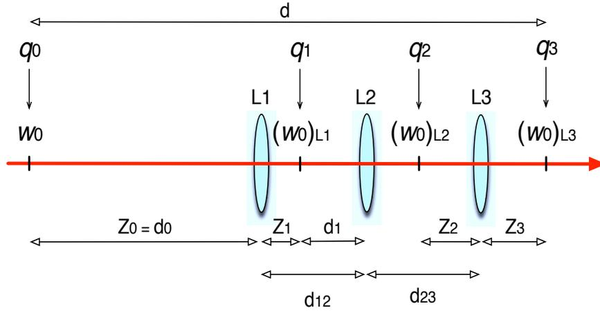
Figure 8.19: Layout of the  $LG_0^0$  beam mode-matching telescope.
