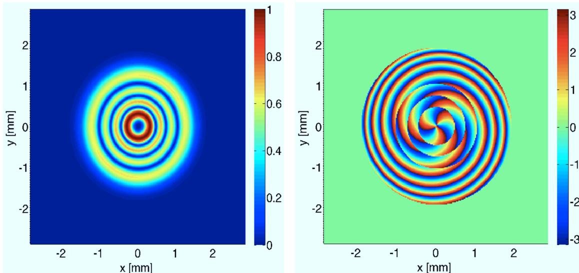
Figure 8.12: Filtered pseudo-LG<sub>3</sub><sup>3</sup> beam transmitted through the mode-cleaner, for  $\mathcal{F} = 100$ : normalized amplitude [a.u.] (left) and phase [rad] (right).
