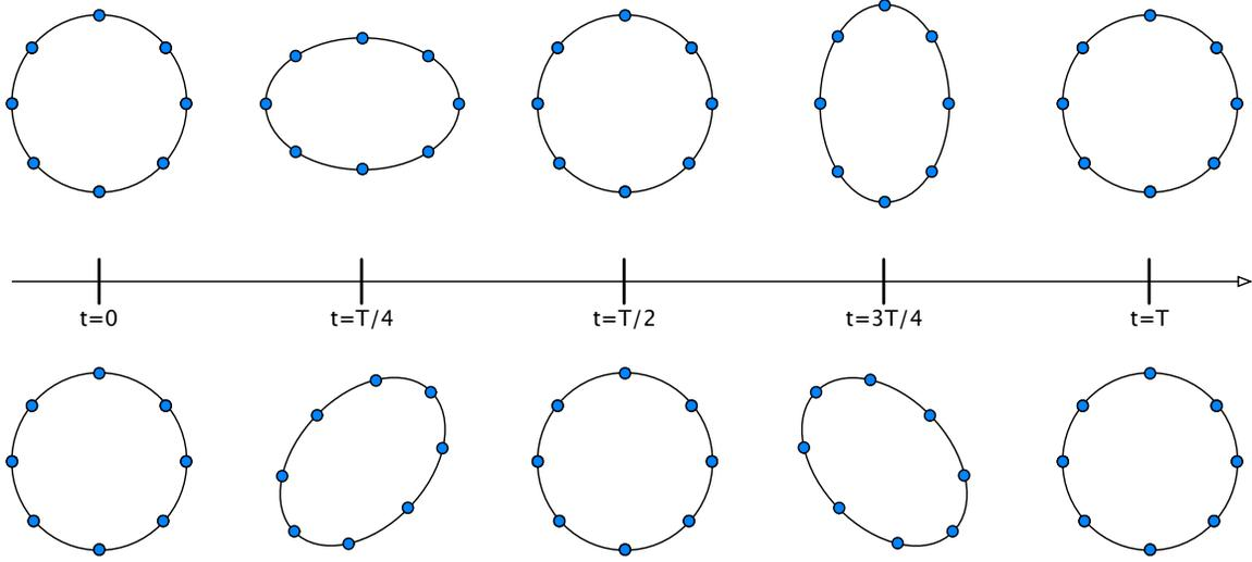
Figure 2.1: Effect of + (top row) and  $\times$  (bottom row) polarized gravitational waves propagating along the  $z$  axis on a ring of free falling masses in the  $x - y$  plane. The strain is shown every quarter of wave period  $T$ .
