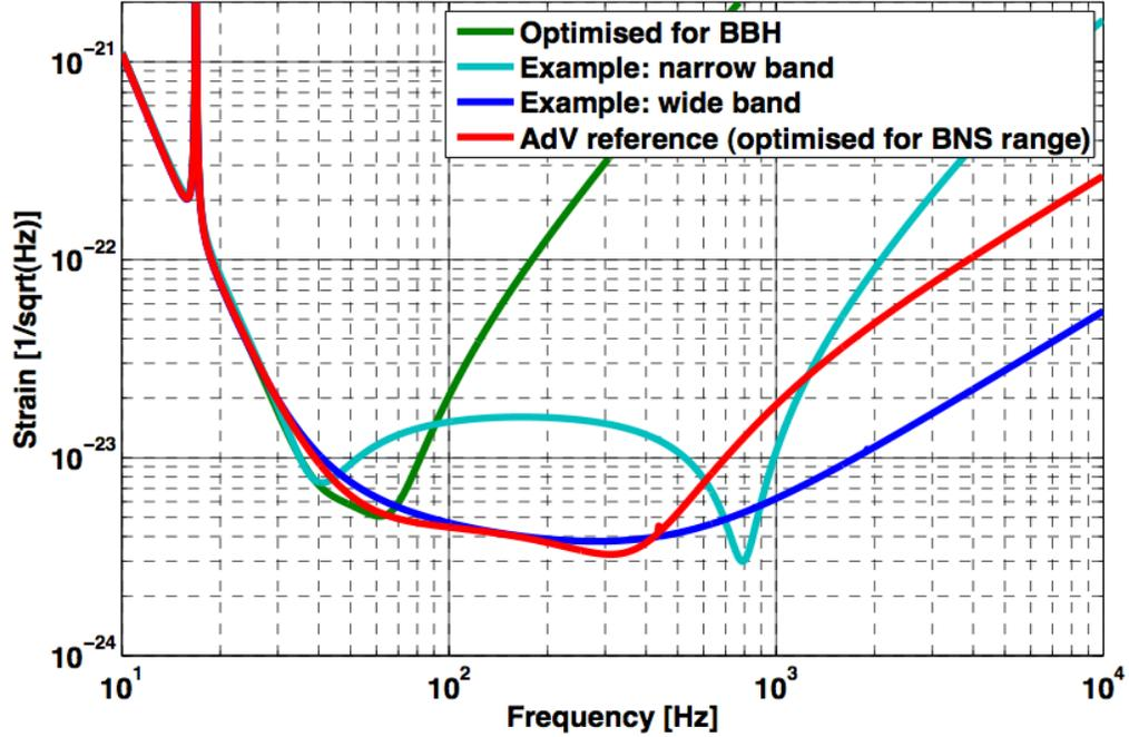
Figure 3.7: Tuning of the sensitivity curve of Advanced Virgo (red curve), from [69]. Maximum detection horizon for black hole-black hole binary systems (green curve), narrow-band tuning for pulsar search (cyan curve), wide-band tuning for burst search (blue curve).
