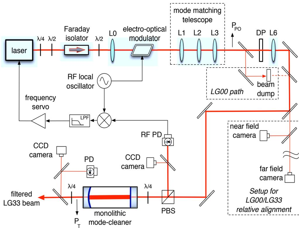
Figure 8.15: Experimental setup for the generating and filtering a pseudo- $LG_3^3$  mode.
