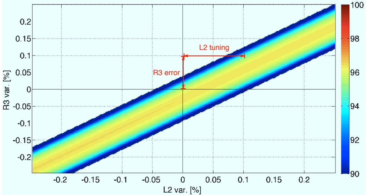
Figure 6.7: Tuning of the lever arm  $L_2$  in the *baseline* design.
