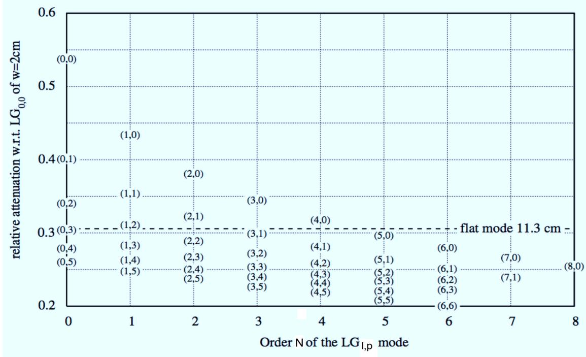
Figure 7.5: Relative reduction of the linear spectral density of mirror thermal noise versus the order of the  $\text{LG}_p^\ell$  mode (with  $w$  tuned for 1 ppm diffraction losses), with respect to the configuration of the arm cavity input mirror of initial Virgo ( $\text{LG}_0^0$  with  $w = 2$  cm on a mirror of radius  $a = 17.5$  cm and thickness  $h = 10$  cm). From [125].
