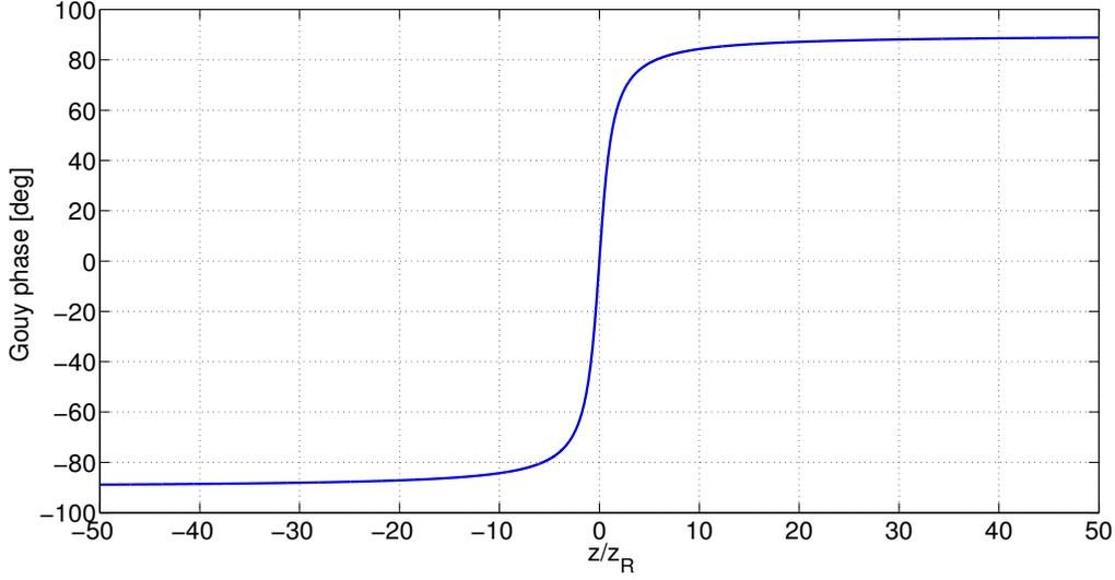
Figure 5.2: Gouy phase shift versus the  $z/z_R$  ratio.
