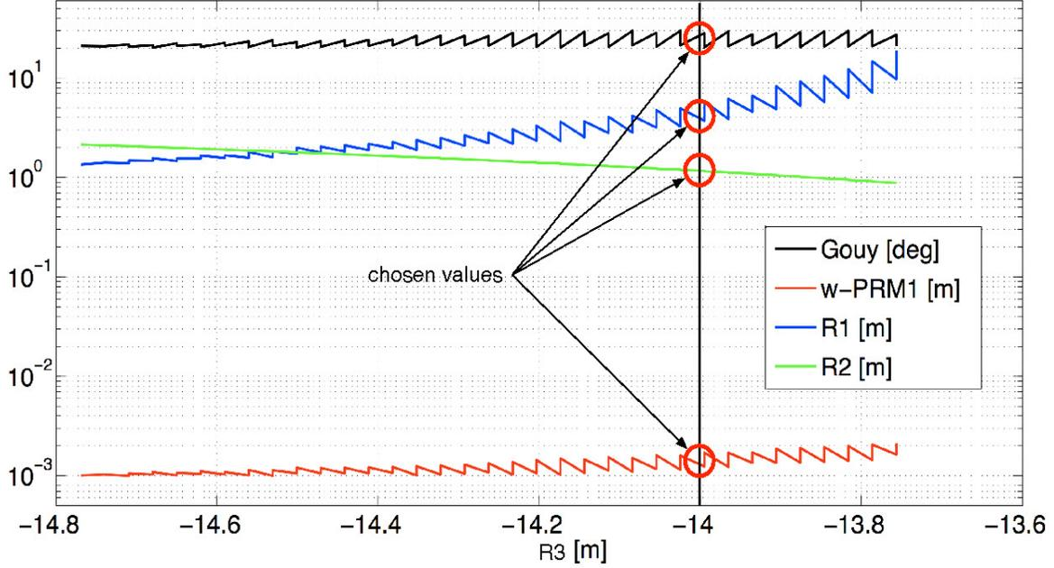
Figure 6.2: Output plot of the space of beam and layout parameters: beam radius  $w$  on PRM1 [m] (red curve), RoC of PRM2 [m] (green curve), RoC of PRM1 [m] (blue curve) and cumulated Gouy phase shift in the cavity [deg] (black curve) versus the RoC of PRM3.
