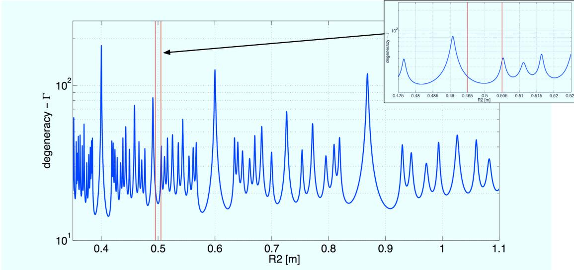
Figure 8.10: Design of the mode-cleaner, choice of the concave mirror radius of curvature: on the  $y$  axis the figure of merit for mode degeneracy (blue line) is shown.  $R = 0.5$  m is the optimal choice, vertical red lines indicate  $\pm 1\%$  mirror manufacturing tolerances.
