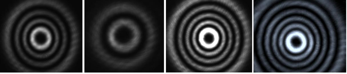
Figure 8.36: Observed mode-cleaner eigenmodes, from the left:  $\text{LG}_1^3$ ,  $\text{LG}_1^l$ ,  $\text{LG}_4^l$ ,  $\text{LG}_5^l$ . Images have been acquired with different filters before the CCD camera, the grey scale is not indicative of the relative intensities of modes.
