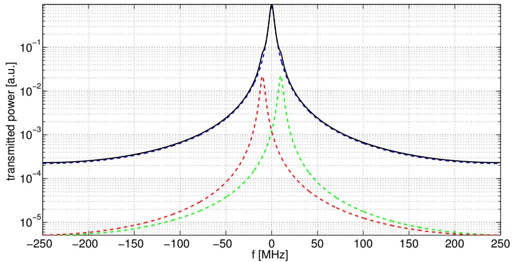
Figure 8.33: Total transmitted field through the  $LG_3^3$  beam mode-cleaner (black solid curve). The carrier field (blue dashed curve), the lower (red dashed curve) and the upper (green dashed curve) radio-frequency sideband fields are shown.
