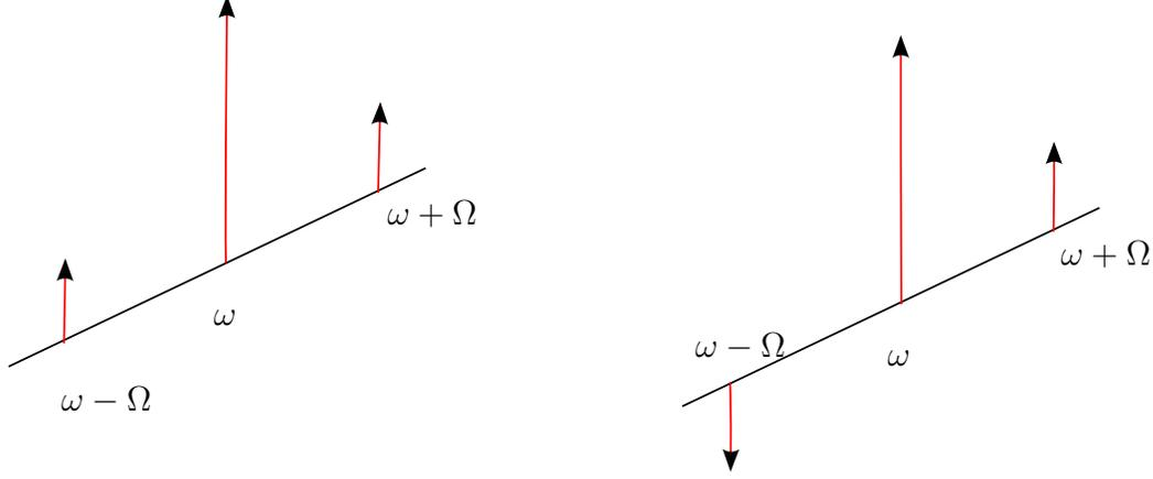
Figure 1-2: Phasors of amplitude noise (left) and phase noise (right) in the sideband picture. In the frame rotating at the carrier frequency  $\omega$  the carrier is still in these diagrams while the sidebands rotate at  $\Omega$ , the signal at  $\omega + \Omega$  rotating clockwise while the idler at  $\omega - \Omega$  rotates counter clockwise. (Sidebands have equal amplitudes)
