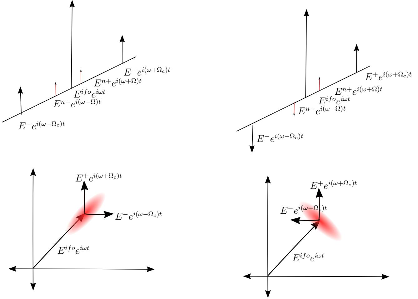
Figure 5-5: Phase relationship between the coherent control sidebands ( $E^+$  and  $E^-$ ) and the local oscillator ( $E^{if_o}$ ), is related to the phase relationship between the noise sidebands ( $E^{n+}$  and  $E^{n-}$ ) and the local oscillator. This means that the coherent sidebands can be used to sense the squeezing angle.
