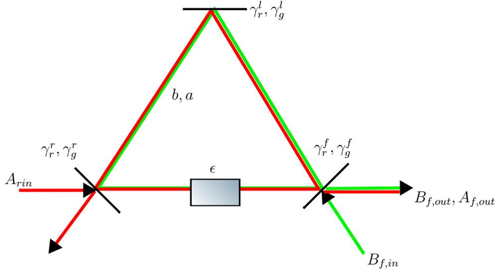
Figure 3-10: Classical OPO with seed. The rear coupler has decay rates  $\gamma_r^r$  and  $\gamma_g^r$ . In Section 2.4 these decay rates were included in the intracavity loss decay rates  $\gamma_r^l$  and  $\gamma_g^l$  but here they will be treated separately.
