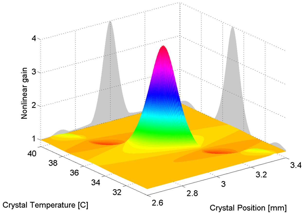
Figure 3-12: Prediction for nonlinear gain as a function of crystal position and temperature for our OPO parameters, and a pump power at one quarter of the threshold value. This pattern is repeated a few times across the width of the crystal, at the same temperatures. The projection on the position axis shows the maximum gain that can be measured at each crystal position once the temperature is optimized.
