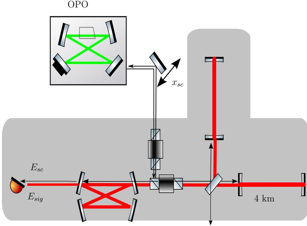
Figure 6-1: Squeezing injected into Enhanced LIGO interferometer. Black arrows represent scattered light,  $E_{sc}$  and  $E_{sig}$  are the amplitudes of the fields due to scattering and the signal field at the gravitational wave readout photo-detector. Path length changes in the scattering path ( $x_{sc}$ ) will add noise to the interferometer's signal.
