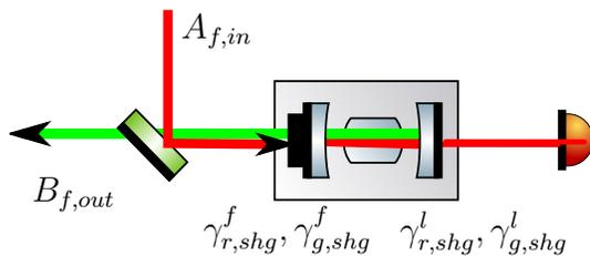
Figure 3-4: Second harmonic generation cavity
