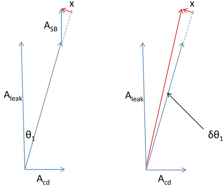
Figure 5-11: Illustration of RF sidebands and contrast defect adding phase noise to the carrier, not to scale.  $A_{cd}$  is the amplitude of the contrast defect light,  $A_{leak}$  is the amplitude of the light due to the interferometer DC offset which is the local oscillator for the self-homodyne used to detect gravitational waves,  $A_{SB}$  is the amplitude of both the sidebands transmitted through the OMC.
