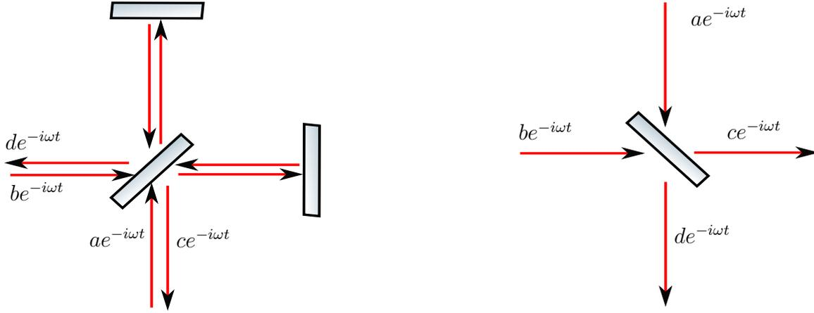
Figure 2-6: Interferometer as a beamsplitter. The main laser input is  $b$ , while the dark port input  $a$  is either vacuum or squeezed vacuum.  $d$  is the reflected field, and  $c$  is the field detected to read out the gravitational wave signal.
