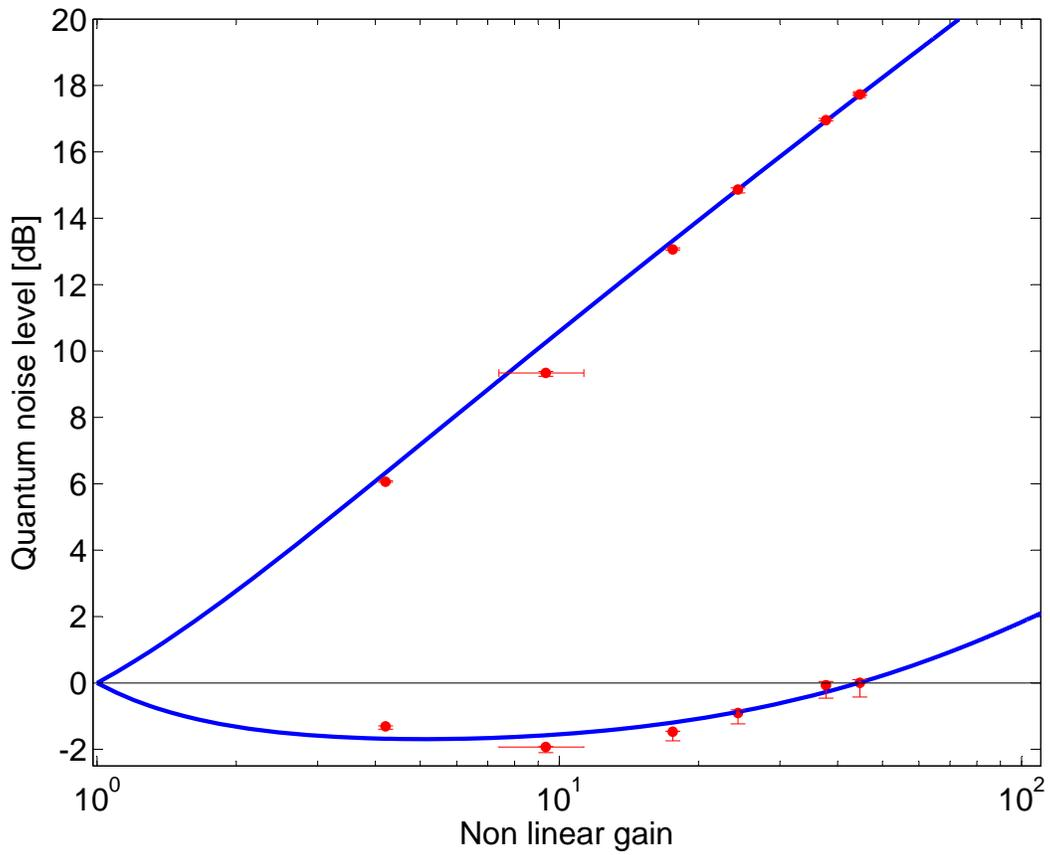
Figure 4-7: Measurement of total efficiency and total phase noise of squeezing during the Enhanced LIGO squeezing experiment. The blue line shows a fit to the red points with total efficiency,  $38.5 \pm 8.3\%$ , and squeezing angle fluctuations of  $81.0 \pm 13.6$  mrad.
