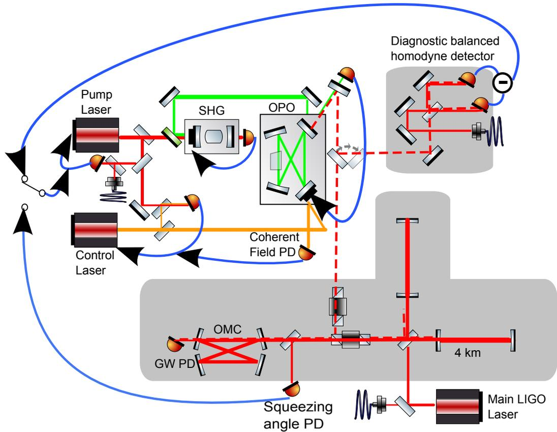
Figure 5-1: Diagram of the control scheme for H1 squeezing experiment
