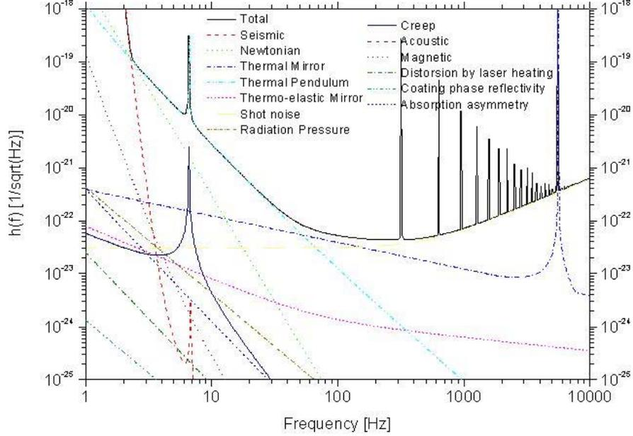
Figure 2.2: *Virgo design sensitivity curve including the noise sources*
