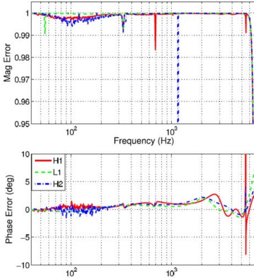
Figure 5.3: *Amplitude and phase systematics as a function of frequency for the three LSC detectors. Blue line in amplitude shows a problem on the H2 detector. Phase error shown in red at 5.5 kHz for H1 indicates a problem with the filters used in the  $h(t)$  production.*
