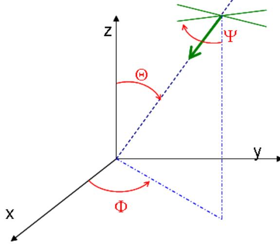
Figure 2.4: Relationship between TT wave frame and detector frame. For an interferometer, the arms are located at the x, y-axis. The angle  $(\theta, \phi, \psi)$  are the Euler Angle of the transformation between detector frame and wave frame.
