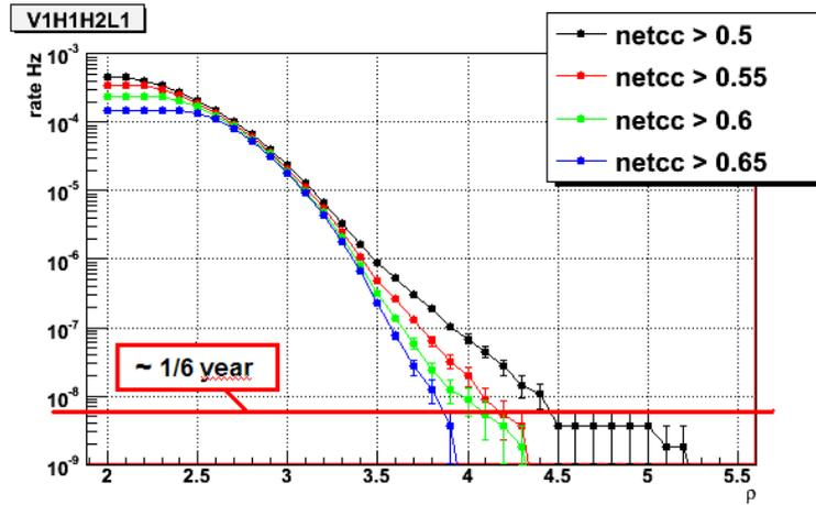
Figure 5.11: Accidental event rate versus  $\rho$  for V1H1H2L1 network. The red line shows the target false alarm rate of  $\sim 1/6$  years.
