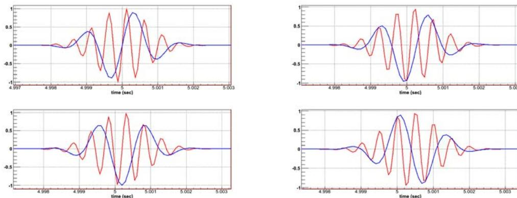
Figure 5.7: *Effect of 5kHz-DC on SG2000Q9. Red is the original signal, blue the down converted one. Signal is arriving at different phase after the buffer center:  $\pi/4$ ,  $\pi/2$ ,  $3\pi/4$ ,  $\pi$  (from left to right, top to bottom). The shape is modified for different phases.*
