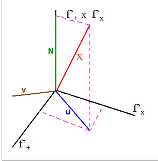
Figure B.1: *Dominant Polarization Frame*,  $v$  is a vector perpendicular to  $u$  in the plane  $(f_+, f_\times)$
