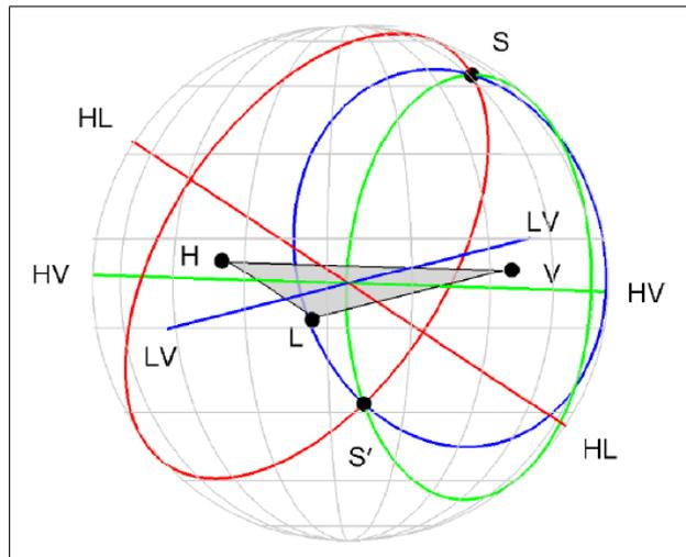
Figure 4.4: *Geometry of the network composed of the three LIGO-Virgo detectors ( $H$ ,  $L$ ,  $V$ ). The locus of constant time delay between two detectors form a ring on the sky concentric about the baseline between two sites. For three detectors, these rings normally intersect in two locations: the source one ( $S$ ) and the mirror image ( $S'$ ). For four or more detectors there is a unique intersection points of all the rings.*
