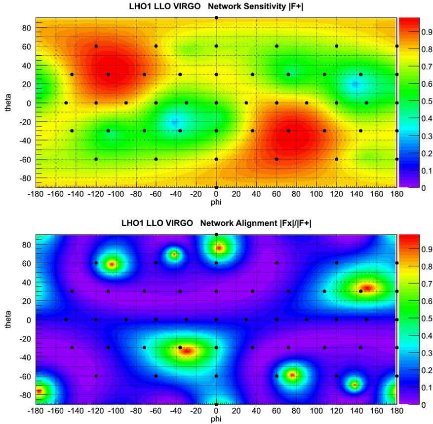
Figure 4.5: *The 46 sky positions chosen for the tests of PRC. Coloured background is  $|f_+|$  (top) and  $|f_x|/|f_+|$  (bottom) values over the sky, where  $f_{+,x}$  are network antenna pattern defined in the Dominant Polarization Frame.*
