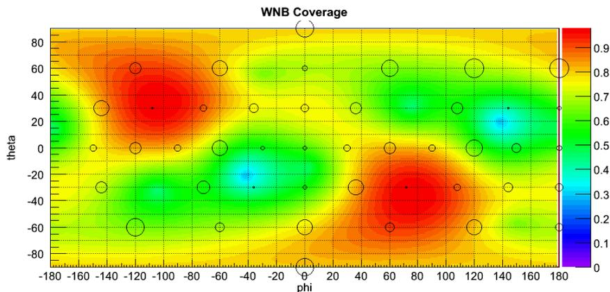
Figure 4.17: *Error Region coverage for the 46 tested sky positions and WNB LF waveform,  $B_{\text{mild}}$  constrain.*
