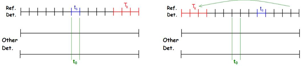
Figure 3.8: Example before (left) and after (right) applying Time Shift on the reference detector (black line on the top). Blue interval is the time step  $t_s$ , red interval is the time shift  $T_k$ . In this case  $k = 3$ .
