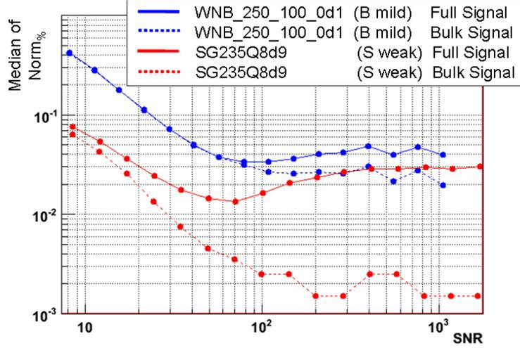
Figure 4.3: Comparison of  $N_{orm}$  for Full (continuous line) and Bulk (dashed line) as a function of SNR for some waveforms with characteristic frequency near 200 Hz. Applied constrains are listed in the figure.
