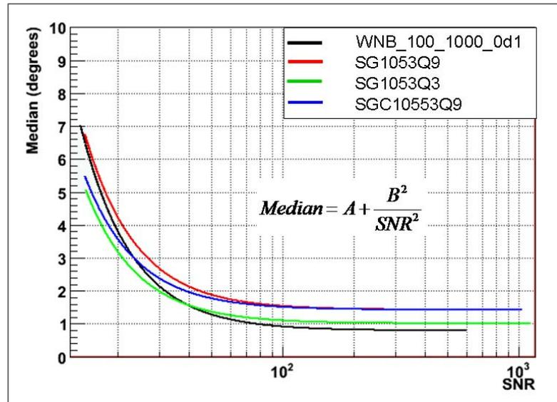
Figure 4.13: *Median  $erA(0)$  as a function of  $\log(SNR)$  for  $Bmild$  search and different HF waveforms: WNB (black), SGQ9 (red), SGQ3 (green) and SGCQ9 (blue). The curves are fitting function following Eq. 4.6*
