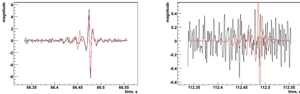
Figure 3.10: *Example of a reconstructed waveform for an event from a background analysis. The red line is the reconstructed signal, the black is the original data. Left: L1 detector, right: V1 detector*
