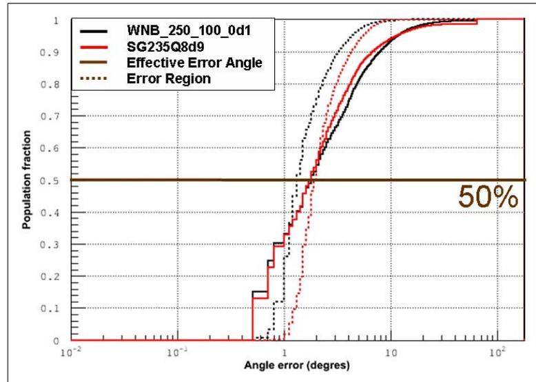
Figure 4.14: *Cumulative curves of Effective Error Angle (continuous) and Error Region (dashed) for WNB and SGQ9 LF waveforms. Bmild search is used for WNB, and Iweak search for SG. Brown line is equal to 50% of y-axis.*
