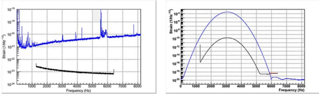
Figure 5.6: *Effect of 5kHz-DC on amplitude for Virgo spectra (left) and SG3067Q9 (right). Blue curve is the amplitude of original data (16384 Hz) applying a Blackman-Harris window, the black curve represents the differences between FFT converted to the sample rate of 10240 Hz and the original one (16384 Hz).*
