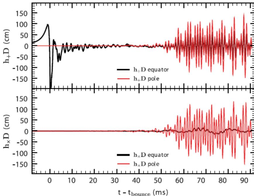
Figure 1.1:  $h_+$  (top) and  $h_\times$  (bottom) multiplied by distance  $D$  as seen by observers along the equator (black) and along the pole (red) of the source for the model  $S20A2B4$  from [20]. Note that the GW burst signal from core bounce is purely axisymmetric, since an axisymmetric system has vanishing  $h_\times$  and vanishing GW emission along the axis of symmetry.
