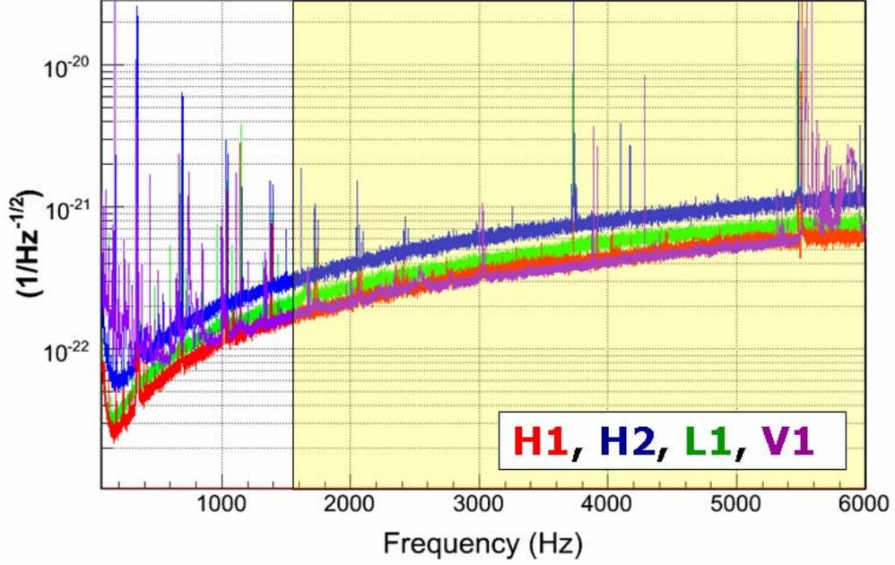
Figure 5.1: *Sensitivity curves for H1 (red), H2 (blue), L1 (green), V1 (purple) during JW1, a week joint period of data acquisition between Virgo and LSC. At 6 kHz the LSC data show some sort of a "cut-off" probably due to the calibration.*
