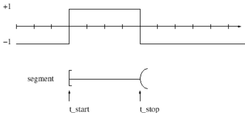
Figure 5.2: *Definition of the segment's boundaries. Starts and stops are respectively included and excluded from the segment.*
