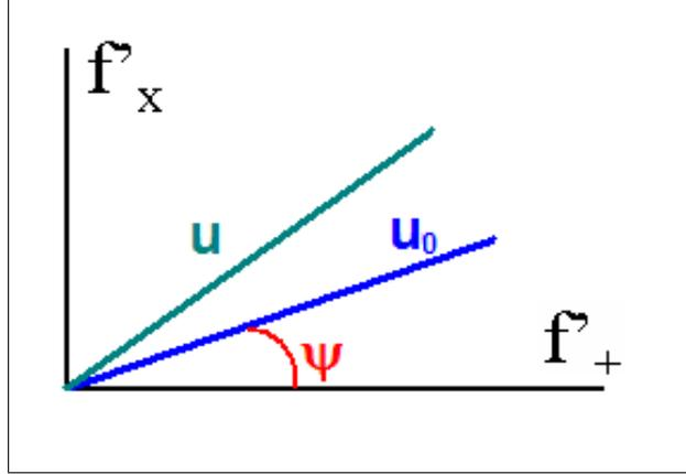
Figure 3.6: Position of the  $u_0$  vector of a regulator and of the associated  $u$  vector given from the minimization of the energy disbalance,  $\psi$  is the angle between the vector and the  $f'_+$  axis.
