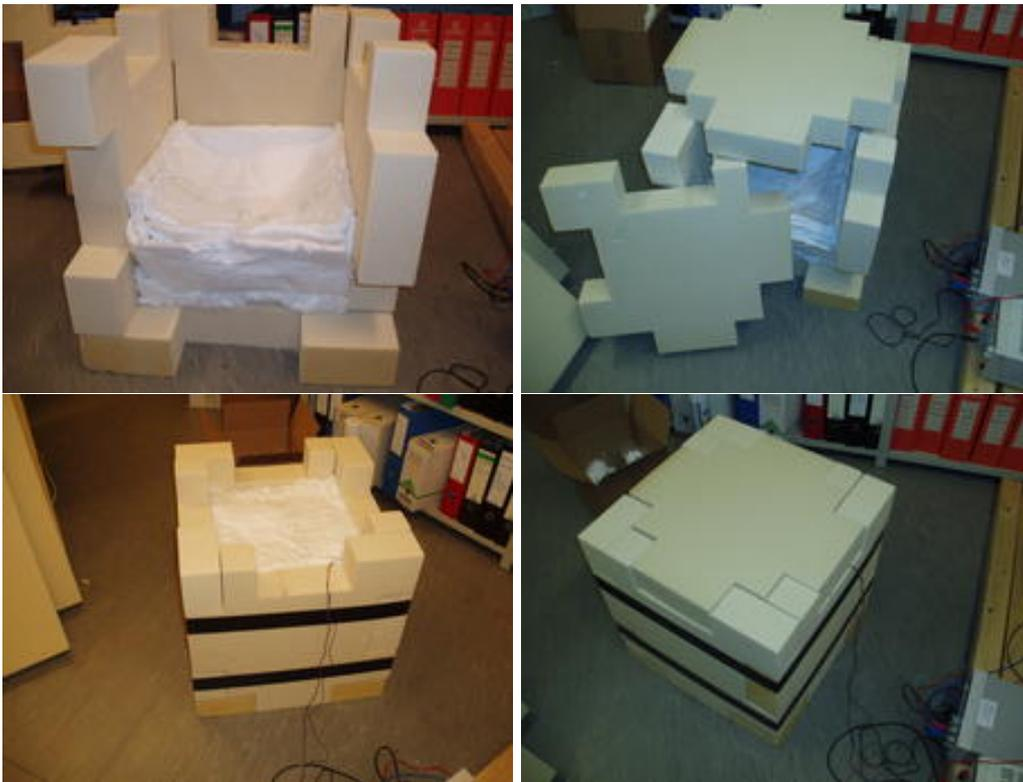
Figure E.2: Construction of the insulator.
