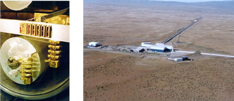
Figure 2.2: **GW Detectors.** The left panel shows the ALLEGRO bar detector at Luisiana, US (image taken from “ALLEGRO Archive Photos” [18]). The right panel shows an aerial view of the LIGO detector at Hanford, US. This instrument, in fact, hosts two detectors of 4km and 2km arms (image taken from “LIGO Press & Media Kit: LIGO photos” [19]).
