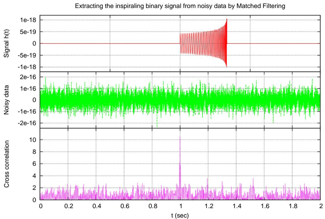
Figure 3.1: **Illustration of Matched Filtering.** Top: Typical “Chirp” signal due to Newtonian compact binaries. Middle: The above signal is injected into comparatively strong detector like noise. Bottom: Matched filtering is done over time of arrival and high correlation is seen when the time of arrival matches the injection time of arrival.
