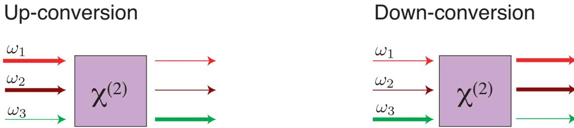
**Figure 3.8:** A representation of different  $\chi^{(2)}$  nonlinear interactions. Left: Up-conversion; Two low energy photons (at  $\omega_1$  and  $\omega_2$ ) are converted into one higher photon (at  $\omega_3$ ). Right: Down-conversion; One high energy photon (at  $\omega_3$ ) is converted into two lower energy photons (at  $\omega_1$  and  $\omega_2$ ).
