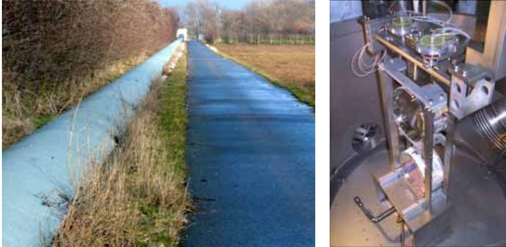
Figure 1.8: *Left: A view along one 600 m long arm of the GEO 600 detector, with the end station housing the end test mass visible in the background. Right: A GEO 600 suspension, consisting of a triple pendulum, with a monolithic silica lowest stage.*
