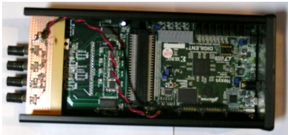
Figure 5.9: Electronics box, shown with frontend based on OPF2416T modules
