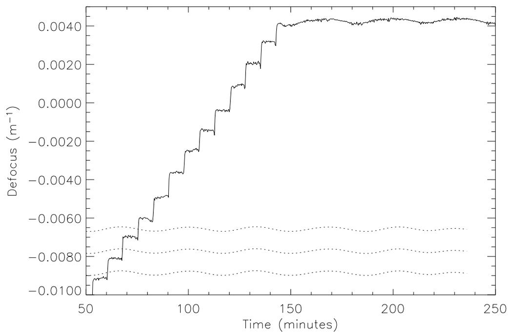
Figure 4.16: The defocus measured by the Hartmann sensor, relative to an average background, versus time where the fibre end is displaced multiple times by approximately  $10\mu\text{m}$  every 7.5 minutes. The dotted lines are sinusoidal curves that have the same frequency and phase as the cyclic fluctuation of the laboratory temperature and are traced backward in time. Notice that the displacement at 68 minutes coincides with a peak.
