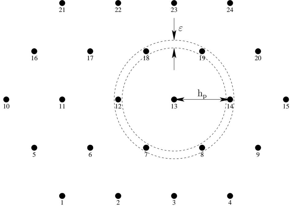
Figure 3.19: Hartmann spots arranged in a hexagonal grid and numbered from 1 to 24. The nearest neighbours of the 13<sup>th</sup> spot are those lying within the dashed annular region of inner radius  $h_p - \varepsilon$  and outer radius  $h_p + \varepsilon$ .
