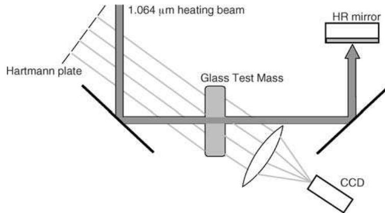
**Fig. 4** A schematic of the off-axis Hartmann sensor.
