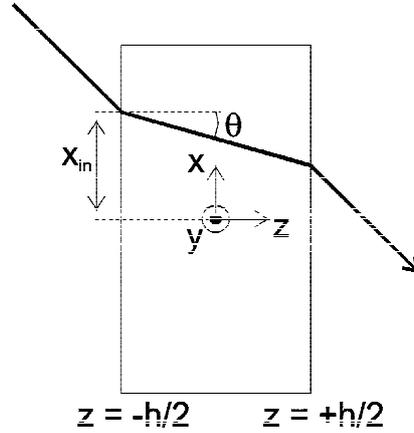
**Fig. 6** The geometry used to determine the expected OPD of a particular Hartmann ray. The ray enters the test mass at  $(x_{in}, y_{in}, z = -h/2)$ . Transverse aberrations are measured in the coordinate frame of the CCD camera and transformed via a suitable rotation into the coordinate frame of the test mass.
