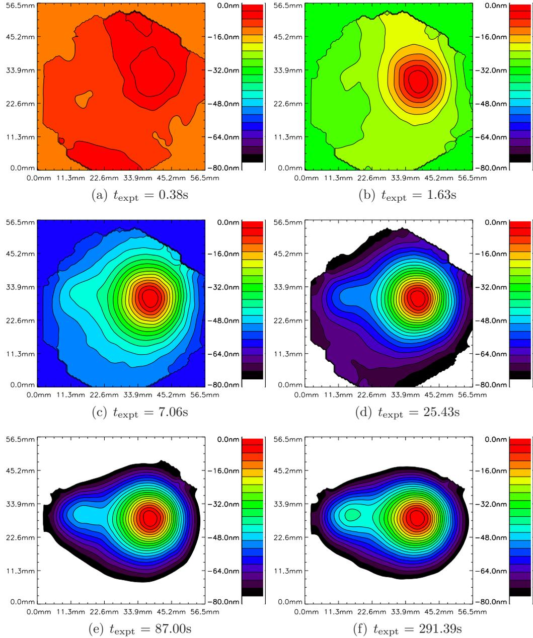
Figure 5.13: Contour plots of the wavefront distortion in sapphire and fused silica,  $\text{WD}^{(\text{off})}$ , at various times from  $t_{\text{expt}} = 0$  s, at which the laser was locked to the cavity. In order to compare the wavefront distortion at different times, all plots share the same colour scale. As such, parts of the distortion saturate the scale at later times resulting in an apparent reduction of spatial extent with time.
