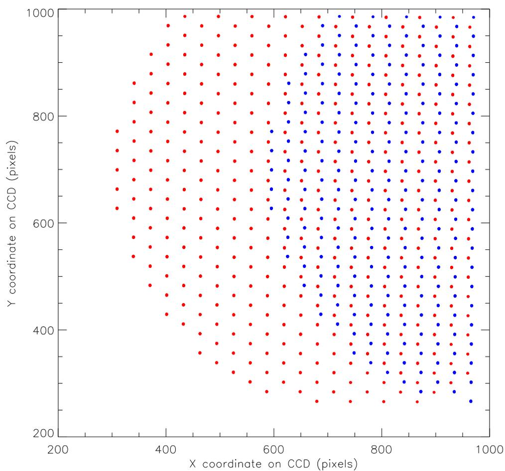
Figure 4.2: The measured centroids on the CCD for the HeNe aligned with needles A and B (red) and with needles C and B (blue). Note that the circular mask was digitally added after the measurement as a visual aid.
