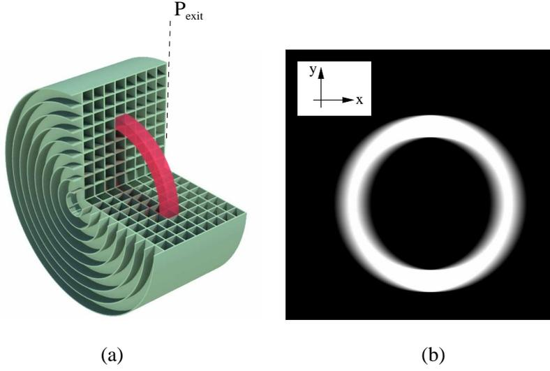
Figure 6.3: a) An example of a single annular volume element,  $V_{ij}(r, z)$ , and b) a grayscale map of the corresponding wavefront distortion,  $w_{ij}(x, y)$ , measured at the exit plane,  $P_{\text{exit}}$ .
