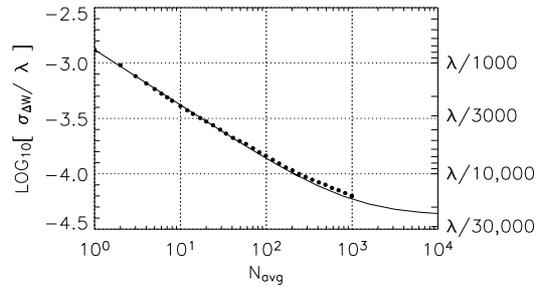
Fig. 3. The improvement in H-WFS sensitivity due to averaging over  $N_{\text{avg}}$  Hartmann images. The solid curve shows the improvement predicted by a numerical simulation assuming only random, stationary noise in the spot centroids.
