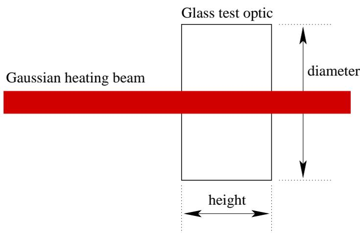
Figure 2.1: A cylindrical test optic exposed to a Gaussian beam expected to absorb optical power in the substrate and produce a wavefront distortion as described by Hello and Vinet
