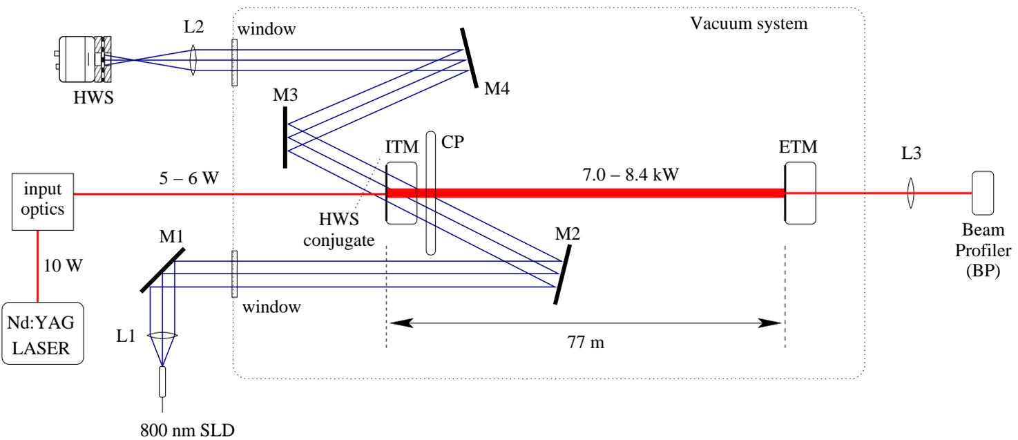
Figure 5.2: Schematic showing HWS installed to measure thermal lensing in the ITM and CP.
