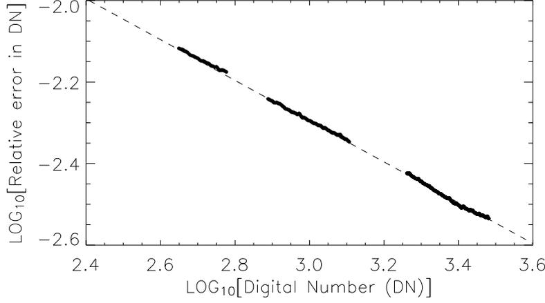
Figure 3.15: RMS fluctuation in intensity vs intensity. The dashed line has a slope of  $-1/2$ .
