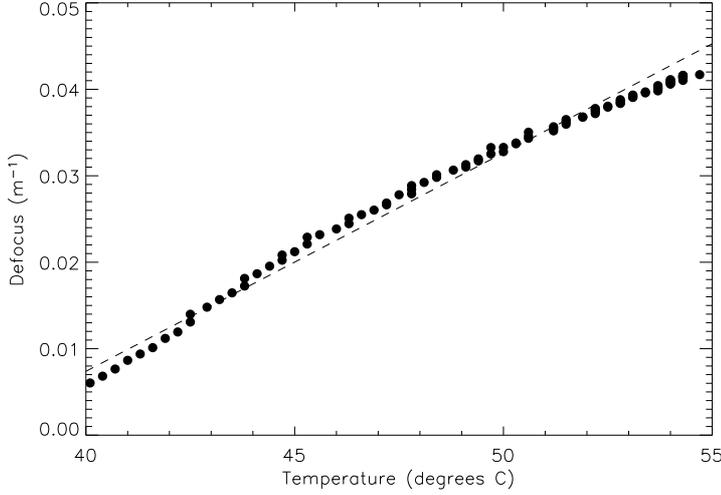
Figure 4.8: Scatter plot of the measured defocus vs temperature. The dashed line is the best linear fit and has a slope =  $0.0025 \text{ m}^{-1} \text{ K}^{-1}$
