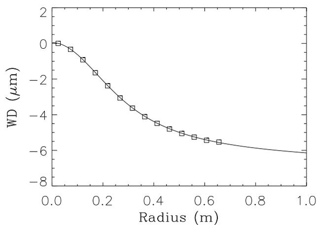
Figure 6.4: Simulation results: a) (left) False colour image of temperature distribution in simulated BG20 glass (arbitrary units) and (right) false colour image of  $14 \times 14$  voxel reconstruction of temperature distribution. Grey area indicates the region not reconstructed. b) Wavefront distortion (WD): directly calculated on-axis distortion,  $WD_{\text{on}}(r)$ , (line) and reconstructed on-axis distortion,  $WD_{\text{fit}}(r)$ , (points).
