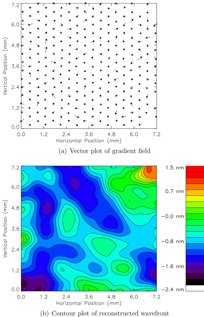
Figure 4.9: Hartmann sensor measurement of the background shot-noise level made by comparing two Hartmann patterns separated in time by approximately 15 s. Shown here are a) the gradient field of the apparent wavefront change and b) a reconstruction of the apparent wavefront change.
