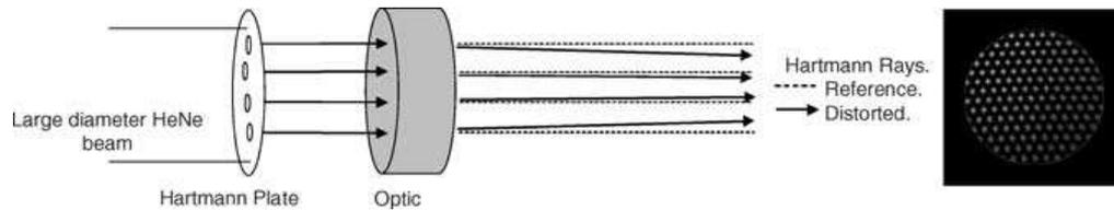
**Fig. 1** A schematic of a prototypical Hartmann sensor. The Hartmann plate contains an array of apertures that produce a set of Hartmann rays. The transverse aberration of the Hartmann rays at the CCD is used to calculate the change in local slope of the wavefront due to the optic.
