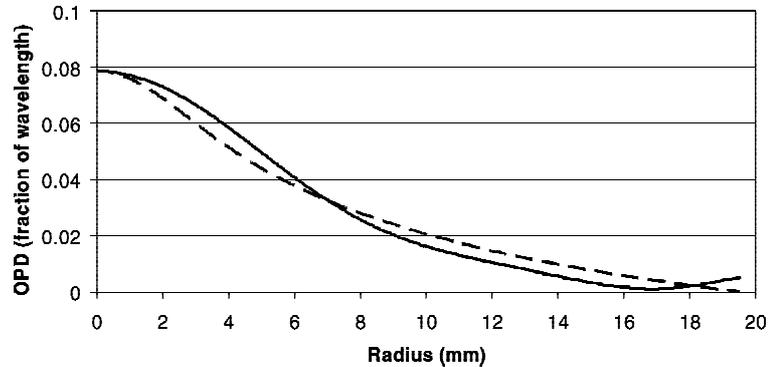
**Fig. 7** A comparison of the wavefront distortion that would be experienced by a laser beam propagating along the axis of the test mass, as determined using the stored-beam interferometer (dashed line) and the off-axis Hartmann sensor (solid line). A HeNe laser,  $\lambda = 632.8$  nm, was used for the measurement.
