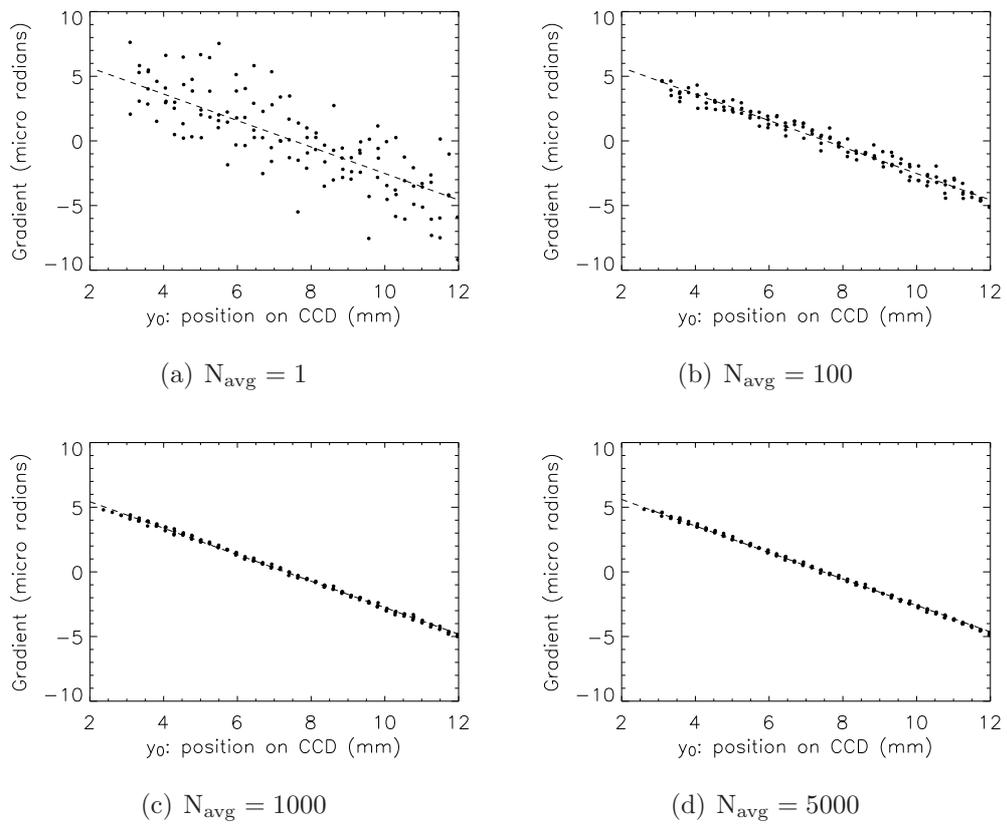
Figure 4.17: Measured local gradient of the wavefront change versus spot position at the CCD,  $y_0$ , due to translation of the fiber light source, averaged over a) 1, b) 100, c) 1000 and d) 5000 Hartmann images.
