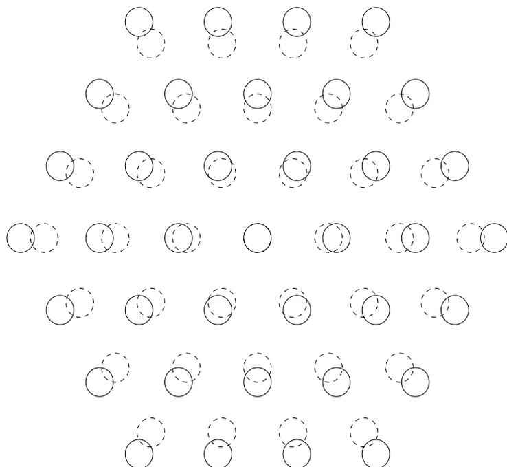
Figure 3.7: Apertures on the Hartmann plate move further apart as the temperature of the plate increases. The dashed circles represent the original positions and the solid circles represent the new positions after an increase in temperature.
