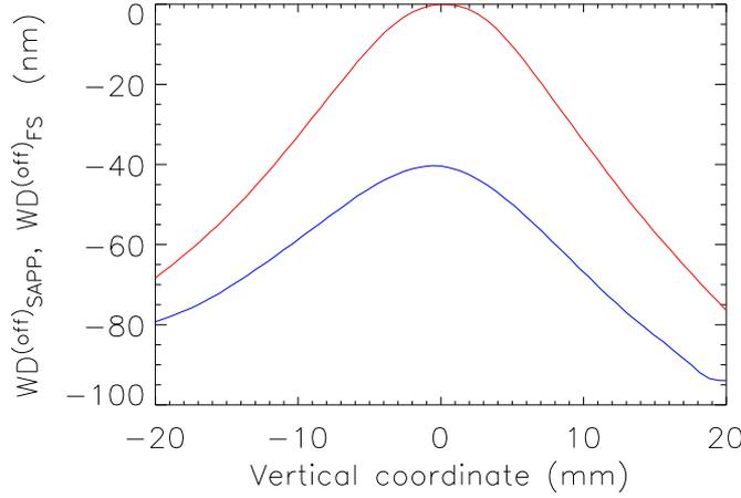
Figure 5.14: Vertical cross-sections of wavefront distortion in the sapphire ITM,  $WD_{\text{SAPH}}^{(\text{off})}$ , (red) and fused silica CP,  $WD_{\text{FS}}^{(\text{off})}$ , (blue). Some residual tilt is present on the WD.
