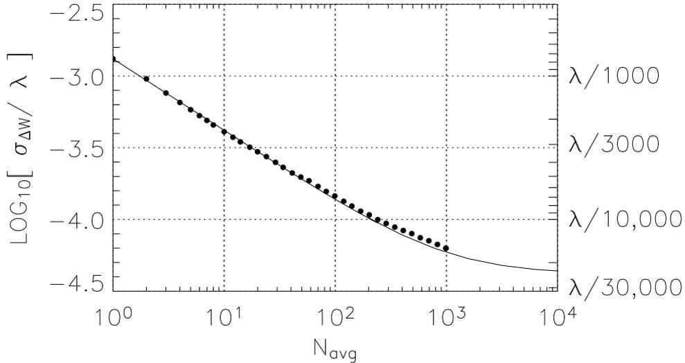
Figure 4.10: The improvement in HWS sensitivity due to averaging over  $N_{\text{avg}}$  Hartmann images. The solid curve shows the improvement predicted assuming only random, stationary noise in the spot centroids
