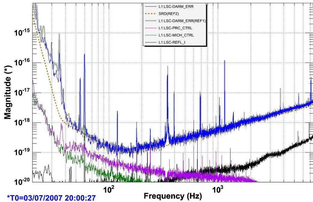
Figure 1.2: The blue curve, L1:LSC-DARR\_ERR, shows the current sensitivity of Initial LIGO in units of  $\text{m}/\sqrt{\text{Hz}}$ , recorded 11th July 2007 at 04:56:07 UTC [9]. The sensitivity is limited by photon shot noise for frequencies  $>$  about 200 Hz.
