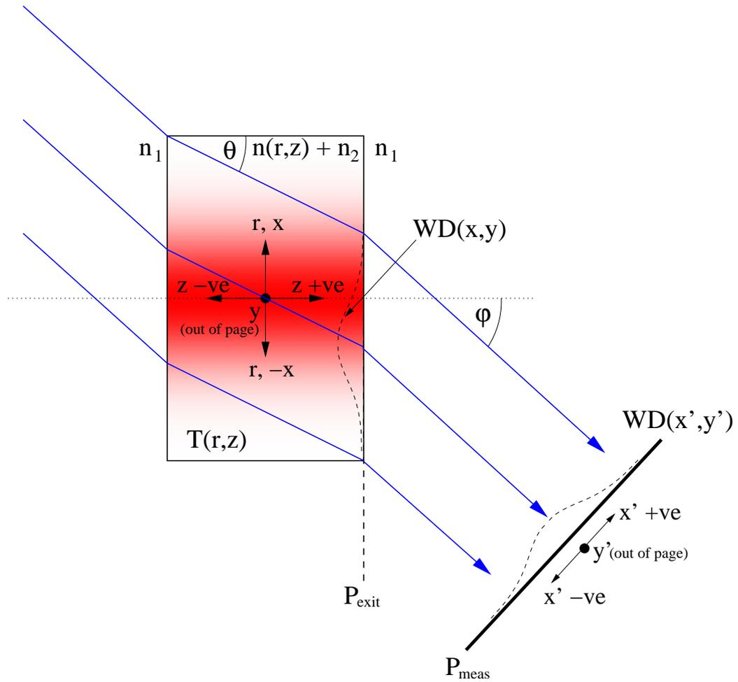
Figure 6.1: Schematic showing off-axis transmission through an axially symmetric thermo-refractive index distribution,  $n(r, z) = dn/dT \times T(r, z)$  in a test optic with nominal refractive index  $n_2$ . The accumulated wavefront distortion,  $WD(x, y)$ , is measured at the plane  $P_{meas}$ . The accumulated wavefront distortion projected onto the exit plane of the optic,  $P_{exit}$ , is denoted  $WD(x, y)$ .
