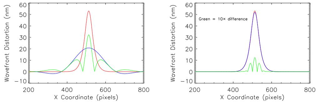
Figure 2.7: a) Image filtering of sharpest H-V signal with bandwidth of 10 spatial frequency unit. b) Image filtering with bandwidth of 70 spatial frequency units. Original signal (red), filtered signal (blue) and a) magnitude of the difference (green) and b) 10× the magnitude of the difference (green). 1 spatial frequency unit =  $1/(1024 \times 1 \text{ pixel}) = 0.0814 \text{ mm}^{-1}$ .
