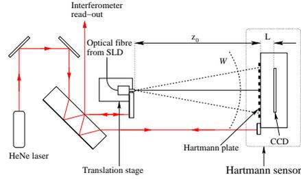
Fig. 1. A schematic of the Hartmann wavefront sensor and the system used to test it. The sensor consists of a Hartmann plate mounted a distance  $L$  from a CCD. It was illuminated by a wavefront  $W$  emitted from a fiber-coupled super luminescent diode (SLD), the free end of which was mounted on a micrometer-controlled translation stage.
