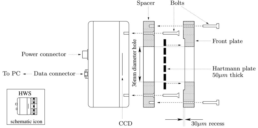
Figure 3.14: A 4mm wide spacer is bolted to the front of the Dalsa 1M60 camera. The Hartmann plate is positioned in a  $30\ \mu\text{m}$  recess in the front plate which is then bolted onto the camera. 36mm diameter holes in both plates allow the the rays to propagate onto the CCD. The inset shows the icon used to represent the HWS in schematic diagrams.
