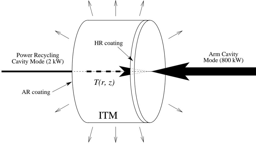
Figure 1.4: Absorption in ITM causes temperature distribution
