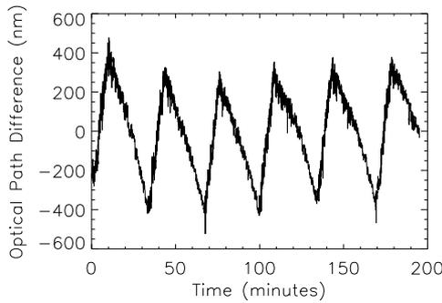
(c) Interferometer measurement
