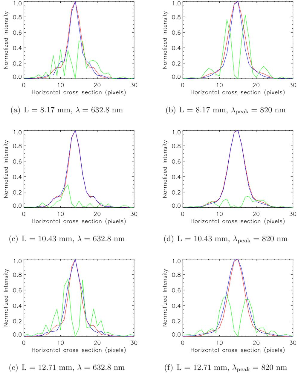
Figure 4.3: Intensity cross sections from measured Hartmann spots (red) illuminated with a), c), e) 632.8 nm coherent light and b), d), f) 820 nm incoherent light. Physical optics simulations by ZEMAX (blue) are also plotted.  $5 \times$  the magnitude of the difference is also shown (green). The best match between measured and simulated is at 10.43mm.
