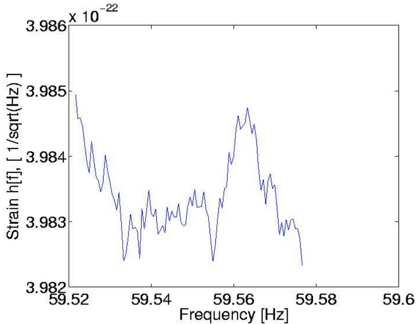
Figure 7-12: Estimate of spectral density of strain versus frequency for the entire Gaussian noise fake data set. This shows the estimation method is working properly, since the estimated strain shown here is within 0.5% of the expected value of  $4 \times 10^{-22}$ .
