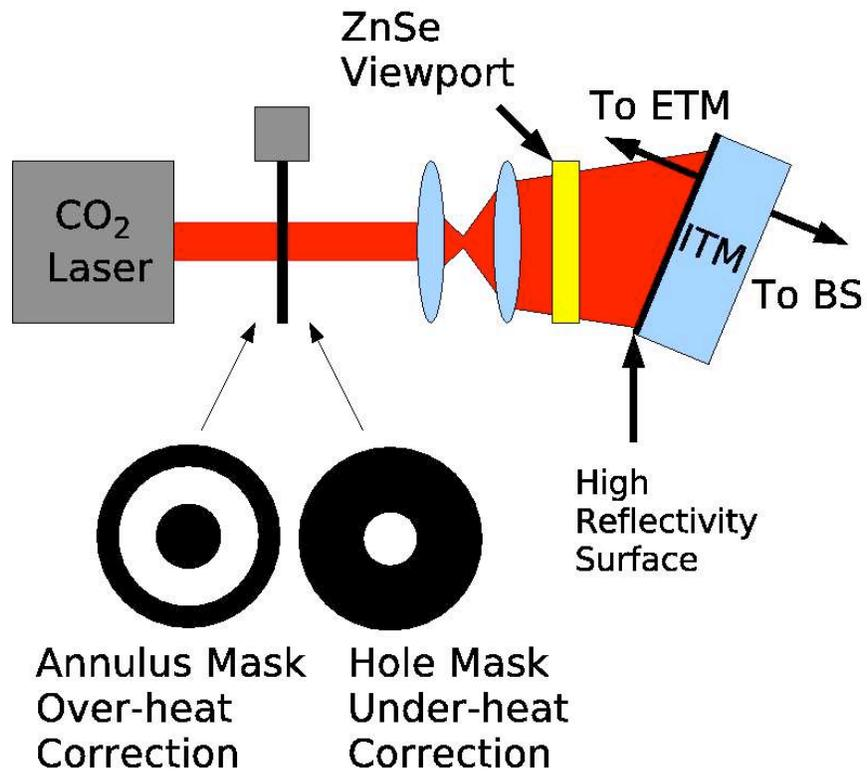
Figure 2-2: A schematic of the Thermal Compensation System (TCS). This was installed on both ITMs on all 3 LIGO interferometers. It is made up of a 10.6  $\mu\text{m}$  CO<sub>2</sub> laser, a set of interchangeable masks, and a series of projection optics that produce an image of the mask on the optic.
