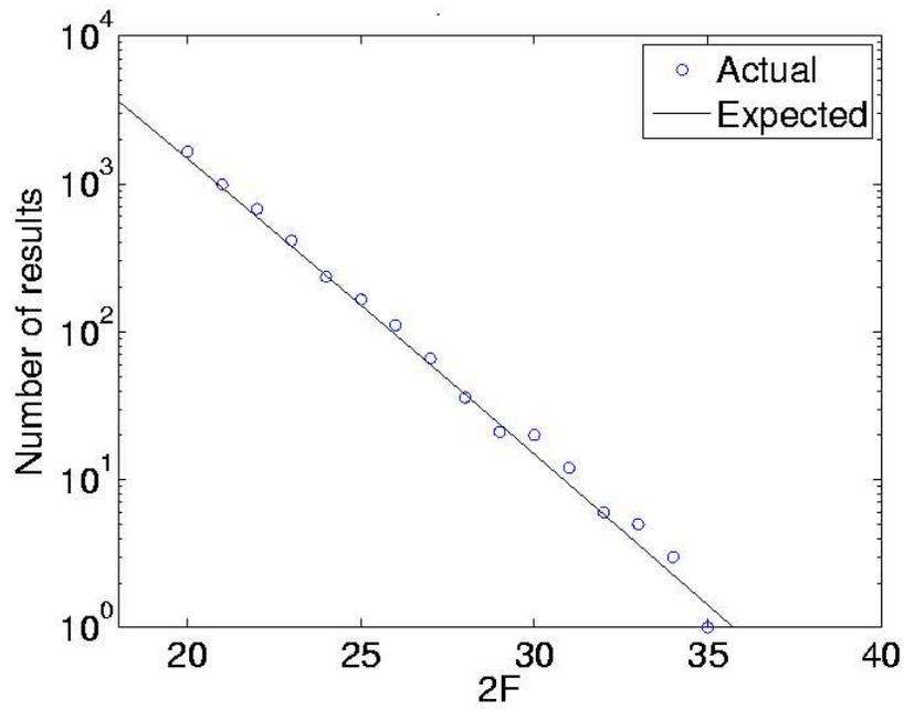
Figure 7-14: Plot of the number of templates returned by a search on a Gaussian noise fake data set with  $2F$  values within a certain band versus the expected number. The fact that the Gaussian noise matches the expected value implies that deviation from the expected in Figure 7-13 for L1 is due to the non-Gaussian nature of the noise rather than a bias in the search pipeline.
