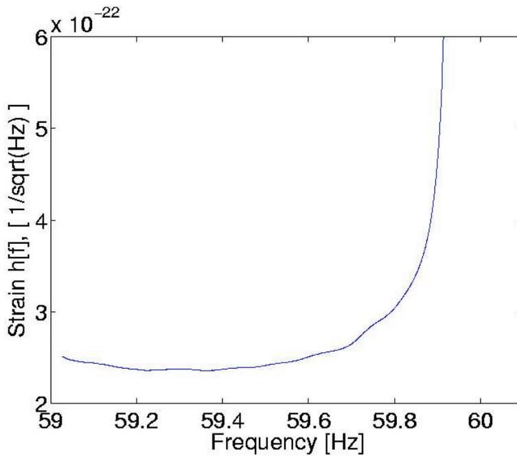
Figure 7-16: Plot of the weighted noise in H1 from 59 to 60 Hz. The really only visible line is the 60 Hz line due to power line noise, while around 59.5 Hz the noise seems effectively flat.
