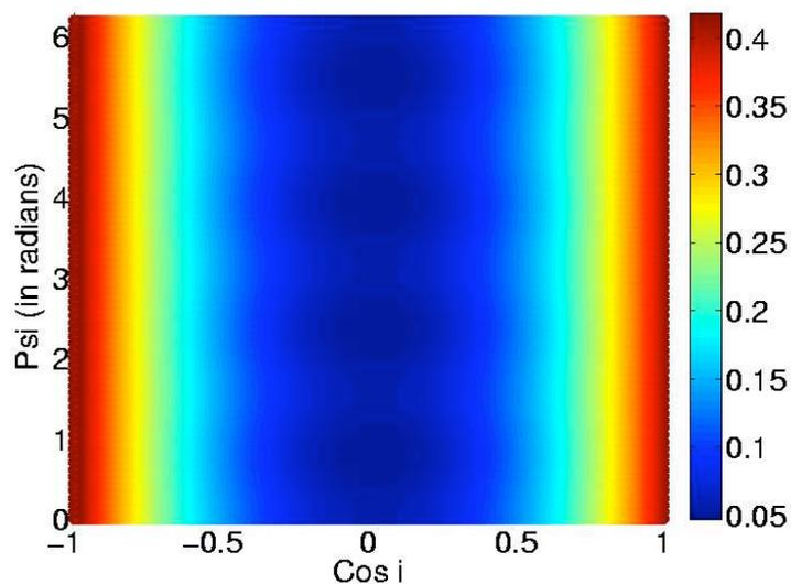
Figure 7-20: Plot of the function  $A(\psi, i)$  for Livingston. Effectively the physical response of the interferometer as a function of the incoming wave's polarization and source inclination, with the sky position fixed to that of the Crab pulsar. Redder colors correspond to higher values of  $A(\psi, i)$ .
