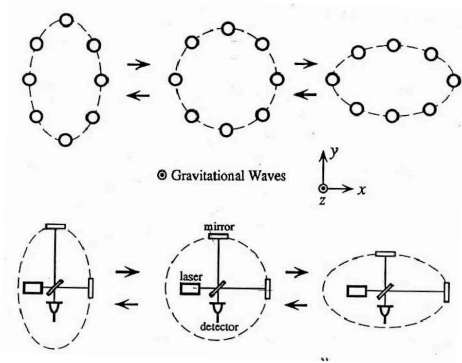
Figure 1-1: Effects of a passing gravitational wave on free masses and a laser interferometer.
