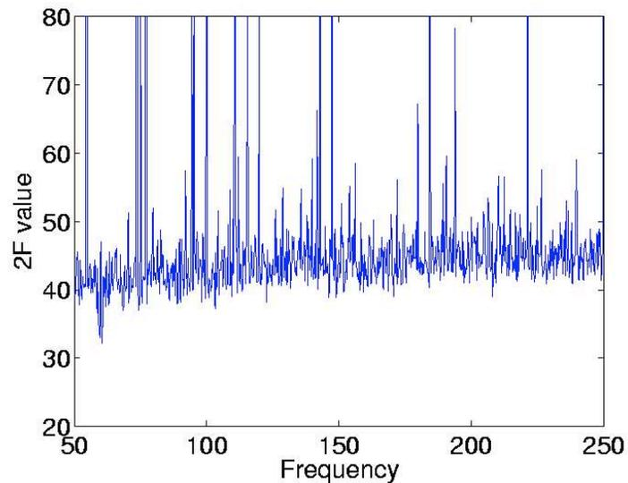
Figure 7-2: Plot of the largest  $2F$  values every 0.25 Hz for the L1 search with the version 1 code. The forest of lines are due to many narrow and strong instrument lines, such as a 37 Hz comb, 60 Hz power lines, and other combs. As in the H1 case, the expected value is roughly 40, increasing at higher frequencies as the number of templates increases per 0.25 Hz band.
