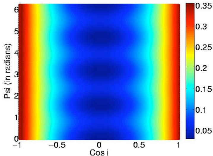
Figure 7-19: Plot of the function  $A(\psi, i)$  for Hanford. Effectively, the physical response of the interferometer as a function of the incoming wave's polarization and source inclination, with the sky position fixed to that of the Crab pulsar. Redder colors correspond to higher values of  $A(\psi, i)$ .
