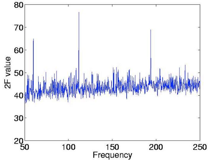
Figure 7-1: Plot of the largest  $2F$  values every 0.25 Hz for the H1 search with the version 1 code. The expected value for any particular 0.25 Hz band is around 40, with slightly higher values expected at higher frequencies because there are more 1<sup>st</sup> spin down values covered and thus more templates searched per 0.25 Hz band. The line at 60 Hz is due to 60 Hz power line noise, the line at 112 Hz is due to a 16 Hz comb, and the line at 194 Hz is due to a hardware injected pulsar.
