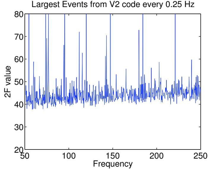
Figure 7-3: Plot of the largest  $2F$  values every 0.25 Hz for the combined H1 and L1 search with the version 2 code. The forest of lines we see is mostly due to the instrumental lines present in L1. The expected value is roughly 40, increasing at higher frequencies due to additional templates searched 0.25 Hz band.
