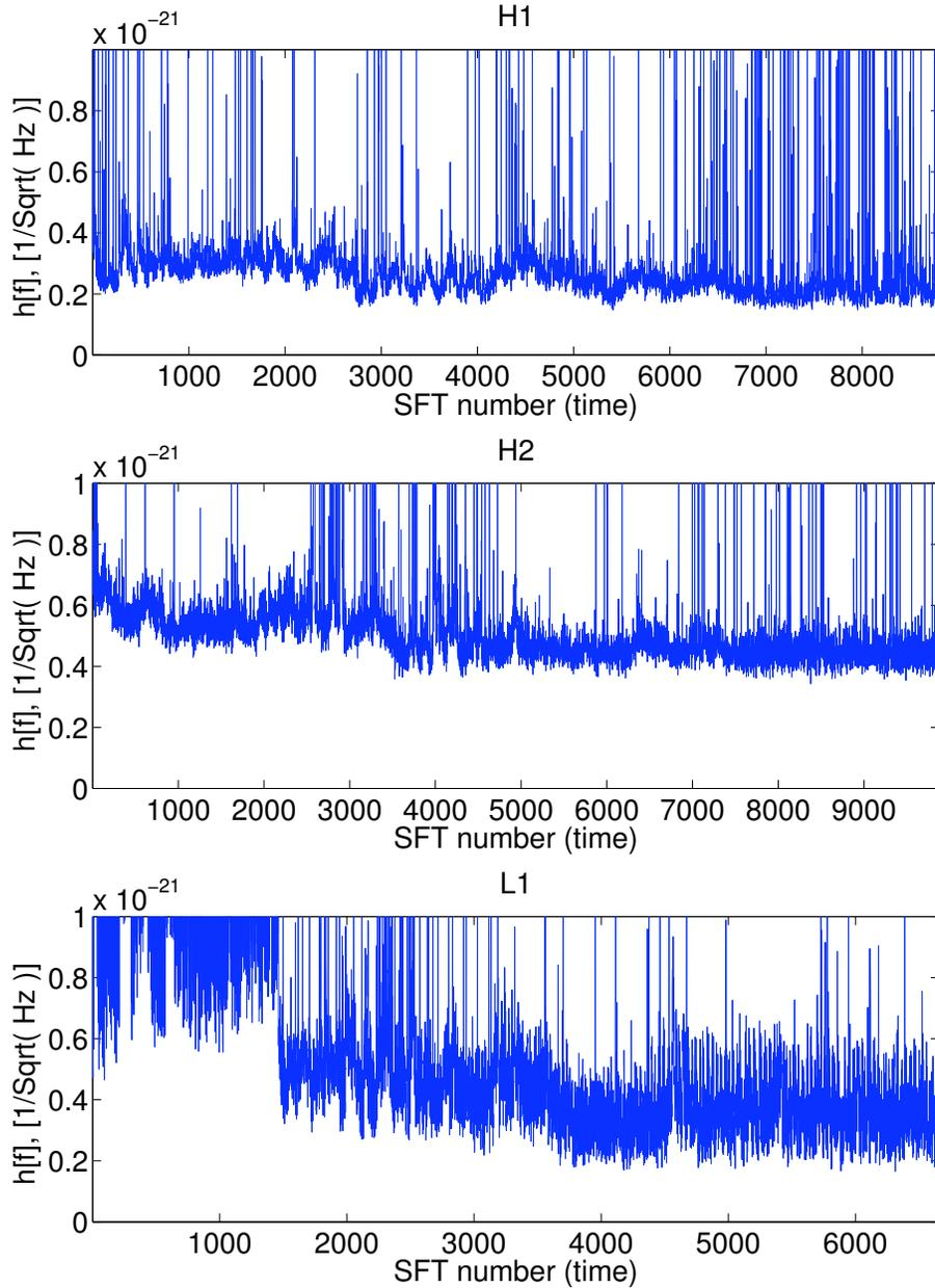
Figure 7-9: Plot of spectral density of strain in the 59.52 to 59.58 Hz band versus SFT (in chronological order) for H1 (top), H2 (middle), and L1 (bottom). The many lines coming out of the noise floor for each interferometer shows the non-stationarity of the noise over the course of the S5 run. In order to get a good estimate of the noise floor a noise weighting scheme is necessary in order to deal with this non-stationarity.
