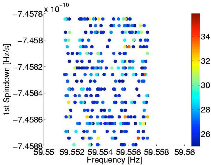
Figure 7-18: Plot of the distribution of  $2F$  values greater than 25 for a Gaussian noise fake data set. The color signifies the  $2F$  value, red is larger and blue is smaller. This is useful as a comparison to the Figures in 7-17 since this fake data set was created without any line or broad spectrum features.
