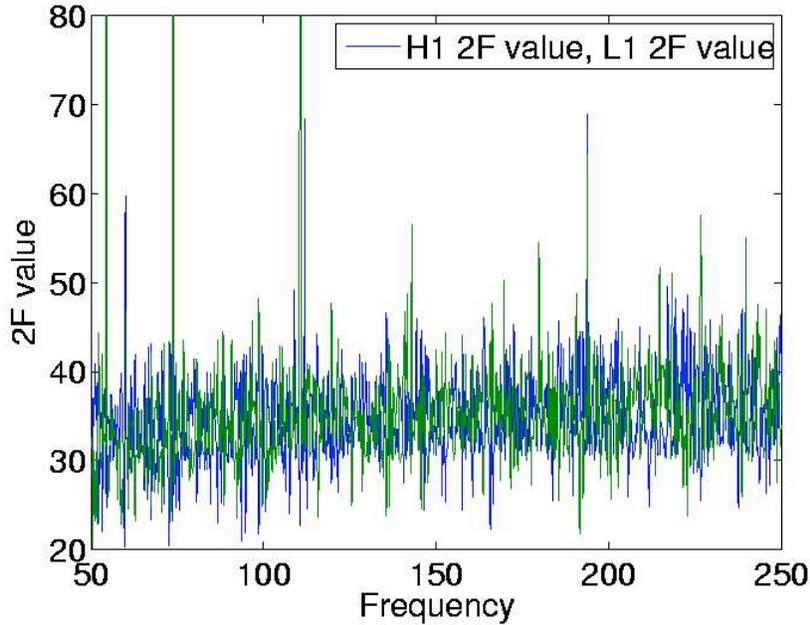
Figure 7-4: Plot of the largest  $2F$  values surviving the coincidence requirement, every 0.25 Hz. There are several lines surviving the coincidence step such as the 60 Hz power line which is present in both interferometers, lines corresponding to a 16 comb, and also with the hardware pulsar injection at 194 Hz.
