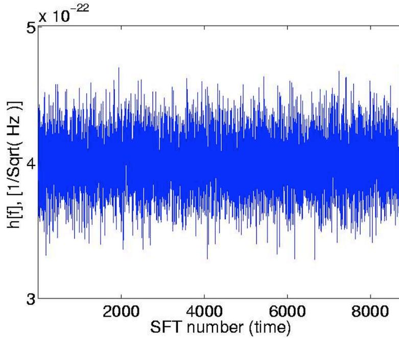
Figure 7-11: Plot of spectral density of strain versus a Gaussian white noise data set SFT (in chronological order). This particular data set has been generated with an expected  $4 \times 10^{-22}$  spectral density of strain.
