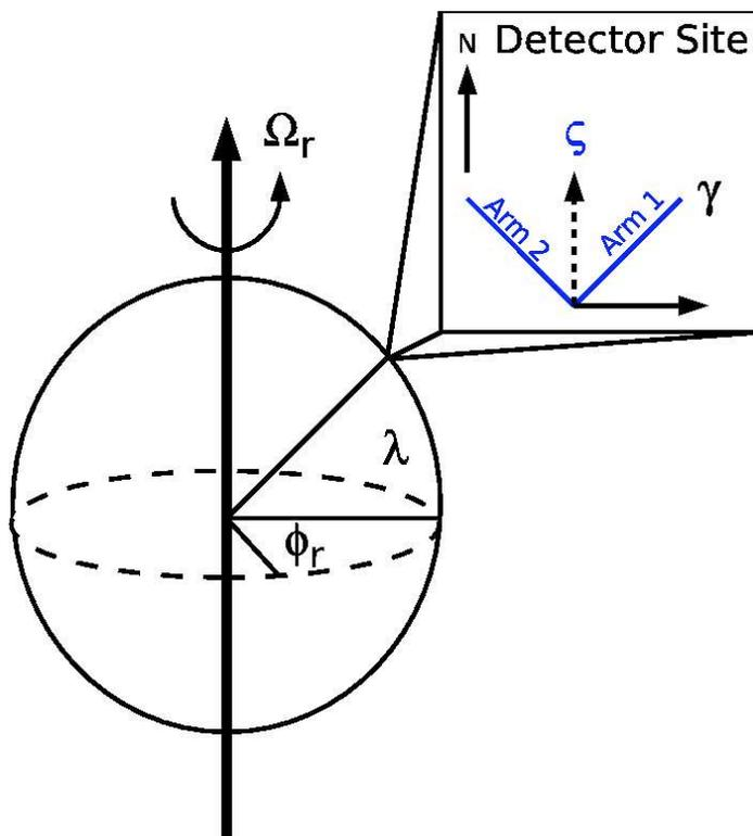
Figure 6-1: Diagram of a Interferometer located on the Earth's surface.  $\Omega_r$  is the Earth's rotation rate,  $\lambda$  is the latitude, and  $\phi_r$  is a reference phase which defines the position of the Earth in its diurnal motion at  $t = 0$ . The inset shows a pair of interferometer arms as if looked down on from above. The angle  $\zeta$  is the angle between the arms ( $90^\circ$  in the case of LIGO) while  $\gamma$  is the angle between East and the arm bisector.
