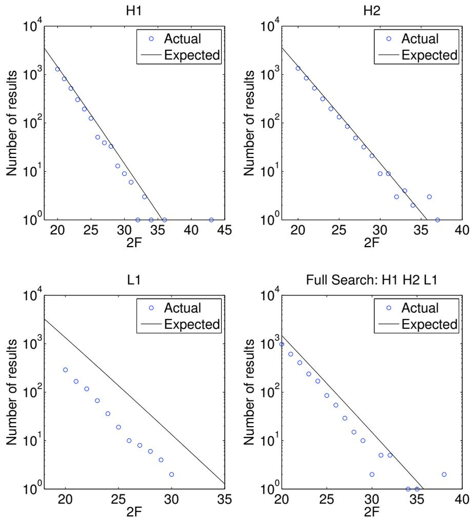
Figure 7-13: For H1 (upper left), H2 (upper right), L1 (lower left) and the full multi-interferometer search (lower right) are shown plots of the number of templates returned by the search with  $2F$  values within a band versus the expected number. In the case of L1 there are far fewer large templates than one would expect primarily due to non-random features in the L1 spectrum. The full search being below expected is mainly due to this disturbance in L1.
