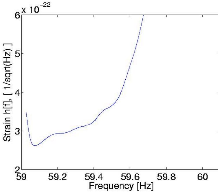
Figure 7-15: Plot of the weighted noise in L1 from 59 to 60 Hz. Distinct steps are visible in the noise, indicating some non-random instrumental effect is raising the noise floor.
